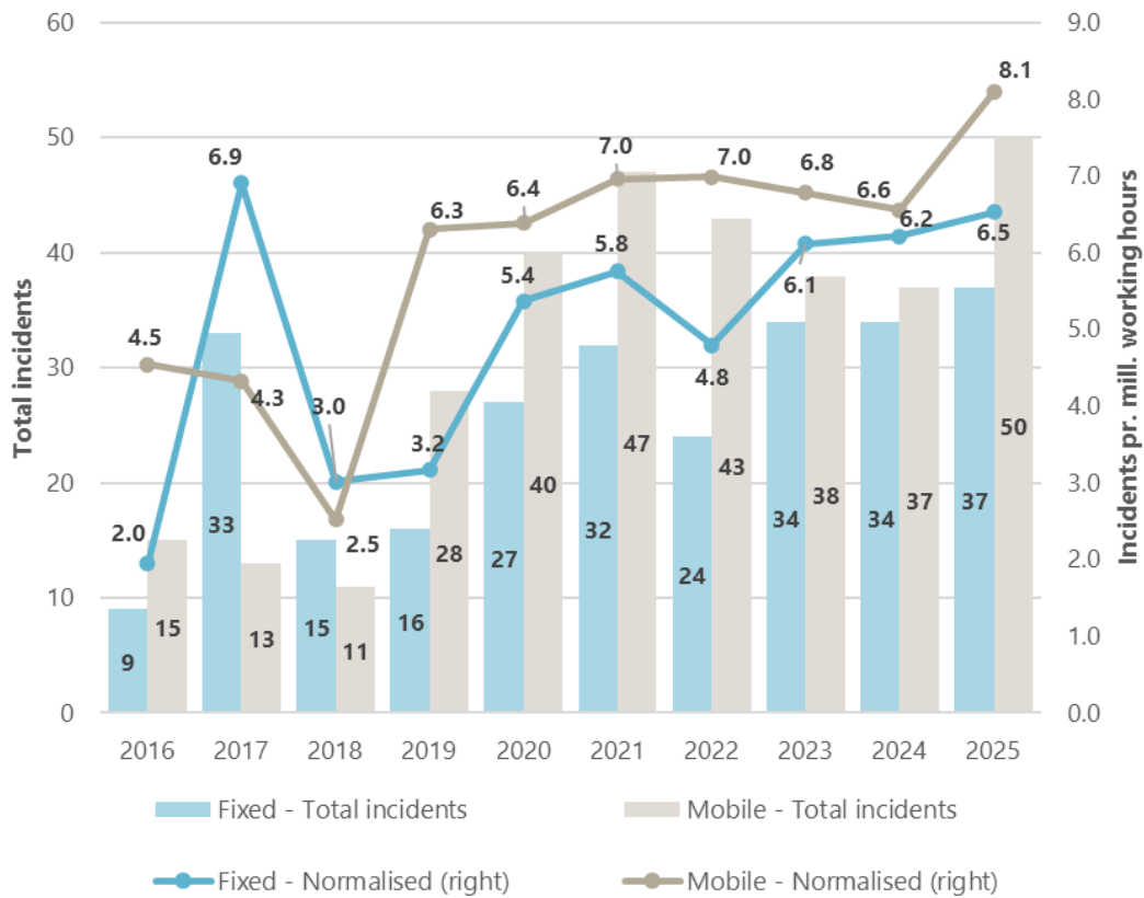
Figure 8-4 Number of incidents related to lifting in drilling module in the period 2016-2025 for fixed and mobile facilities – absolute numbers and numbers normalised against millions of working hours related to (only) drilling and well operations
