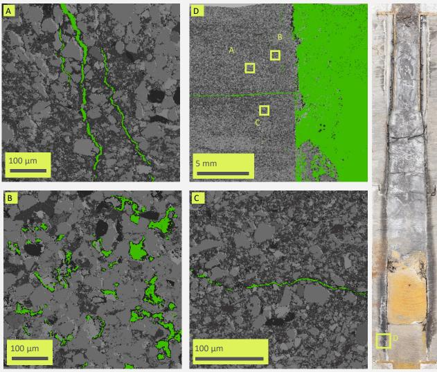
Full Scale Test | 5.5" 17# | Cemented Casing | 7-7/8" Borehole | Mud rock/ Shale Host Rock | 150 bar
