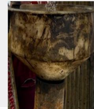
Funnel installed into stick up on drill pipe
