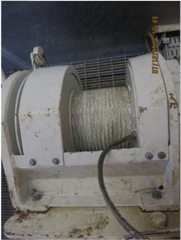
Wire drum on the winch.
