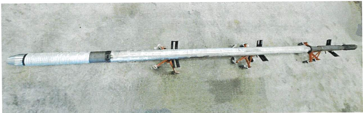
Figure 5 The Bismuth alloy cast on the Wellstrøm running tool
