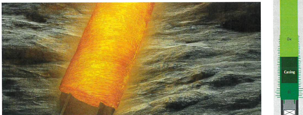
Figure 2 Thermite exothermic reaction and resulting plug, ref. 2
