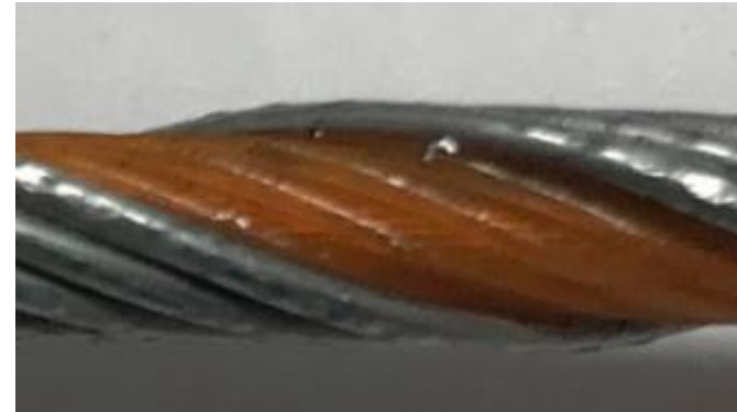
Sealing between armor and insulation
