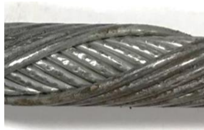
Leak path for gas in between armor
