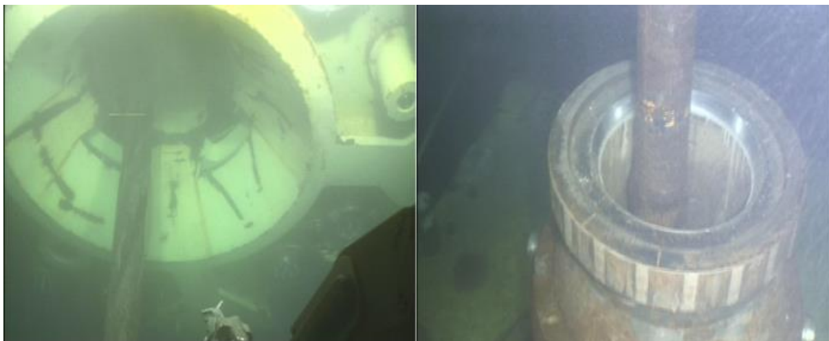
Figure 9: Images taken by ROV after the unintentional disconnection. (Source: Seadrill)
