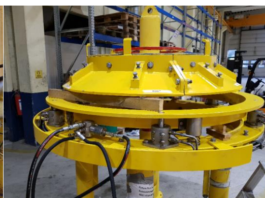
Figure 7: The ADS installed on the West Hercules test bench. (Source: Seadrill)
