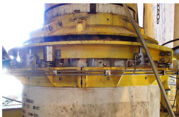
Figure 6: The ADS installed on the West Hercules flexjoint. (Source: Seadrill)
