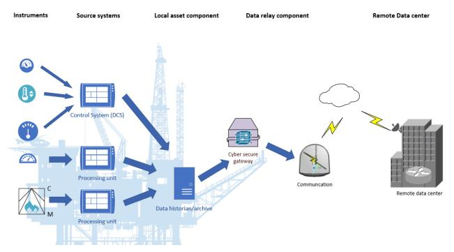
Figure 4-2 Data flow through the sensor system infrastructure
