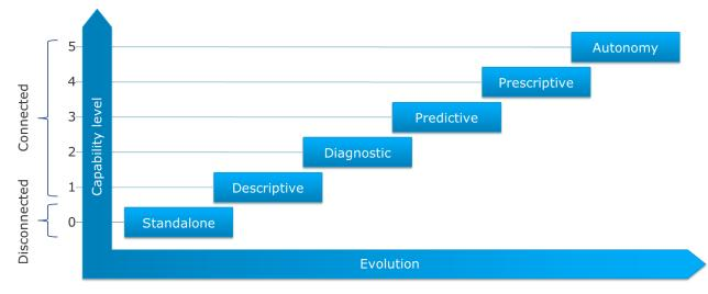
Figure 4-4 Evolution stages or capability levels of a digital twin as presented in DNVGL-RP-A204 /12/.
