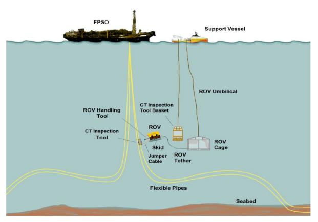
Figure 5-12 Illustration of NDT of flexible riser cross section as presented by Oceaneering /18/
