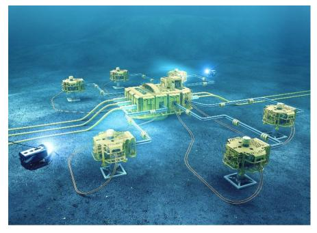
Figure 5-13 SPS illustration. Source: DNV GL
