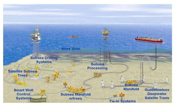
Figure 2-1 Examples of various main systems in a subsea field /5/
