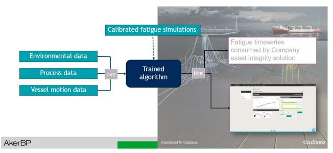
Figure 5-11 Schematic illustrating of flexible riser "Fatigue counter" as presented by 4Subsea /16/, /21/
