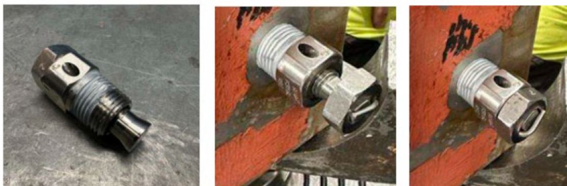
Figure 6 Left: The type of bleed plug used. Centre: The bleed plug in closed position. Right: the bleed plug in open position. Source: Equinor Synergi 2531047 external HC leak in area G.
