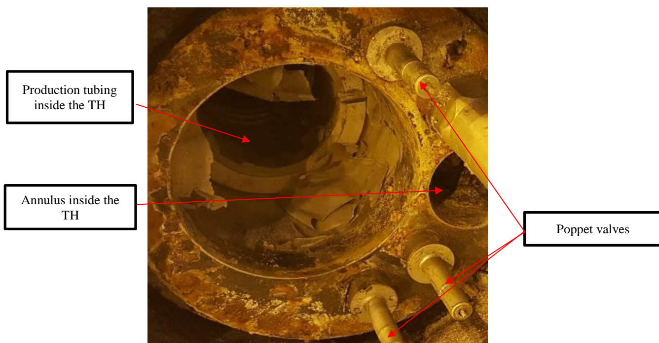
Figure 11 Poppet valves inside the TH. (Source: GE VetcoGray)
