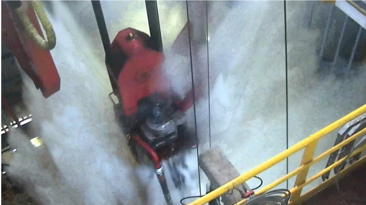
Figure 15 Outflow of gas and fluid at the fingerboard level. (Source: Songa Offshore)
