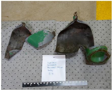
Figure 6: The burst cylinder. (Source: the police)
