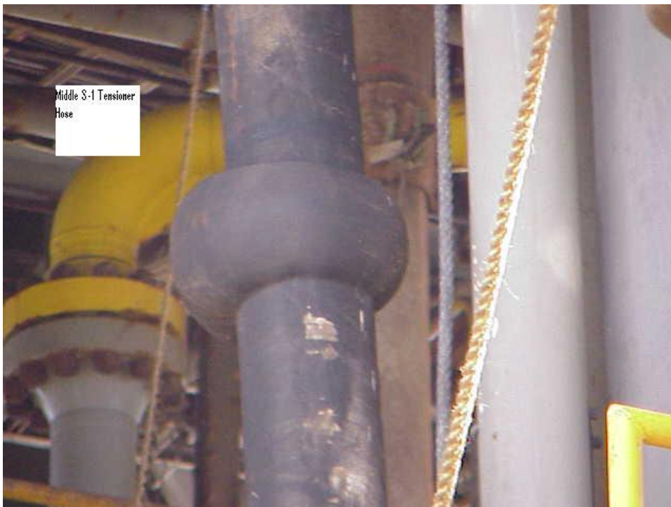
Figure 5.15 Bubble due to absorbed gas, pipe was not designed for gas service, courtesy of Contitech
