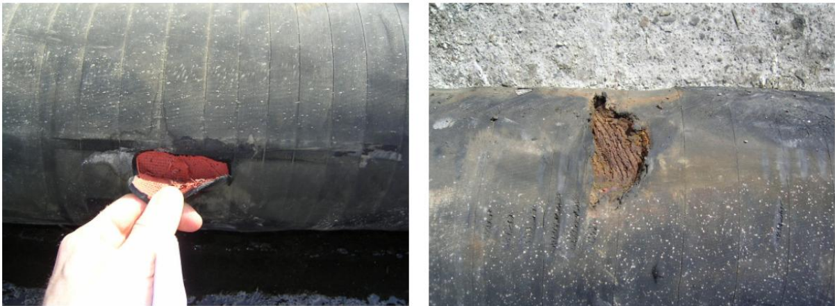
Figure 7.1 Left picture shows repairable damage, right picture is damage beyond repair, courtesy Contitech
