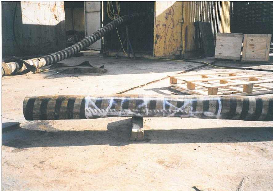
Figure 5.9 Crushing example, courtesy of Contitech
