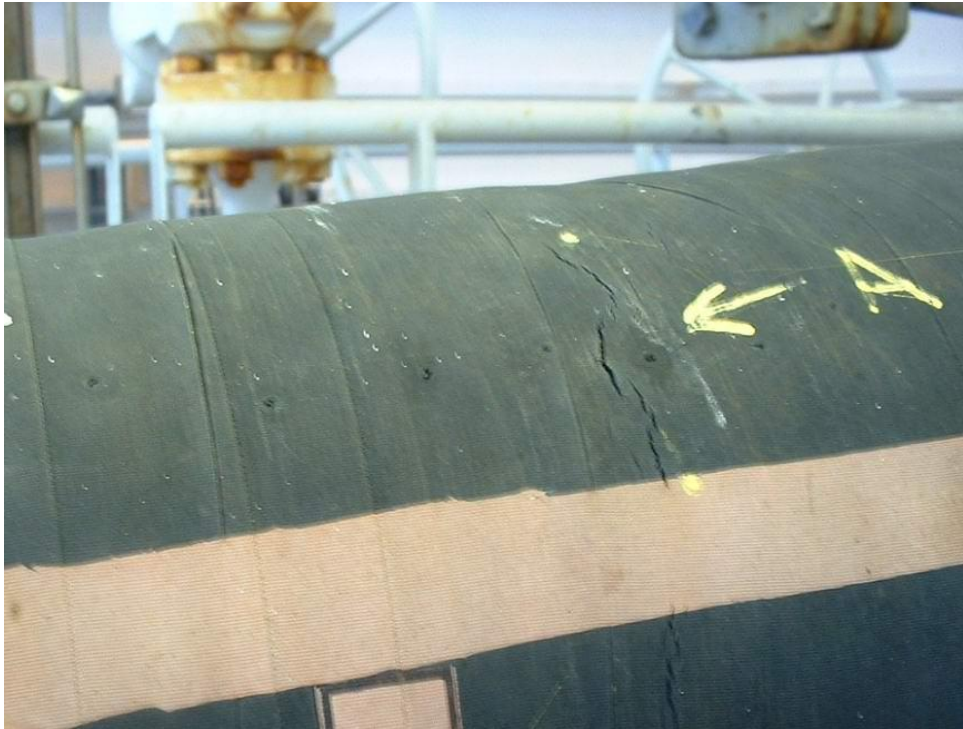
Figure 5.14 Cracking in outer cover, courtesy of Contitech
