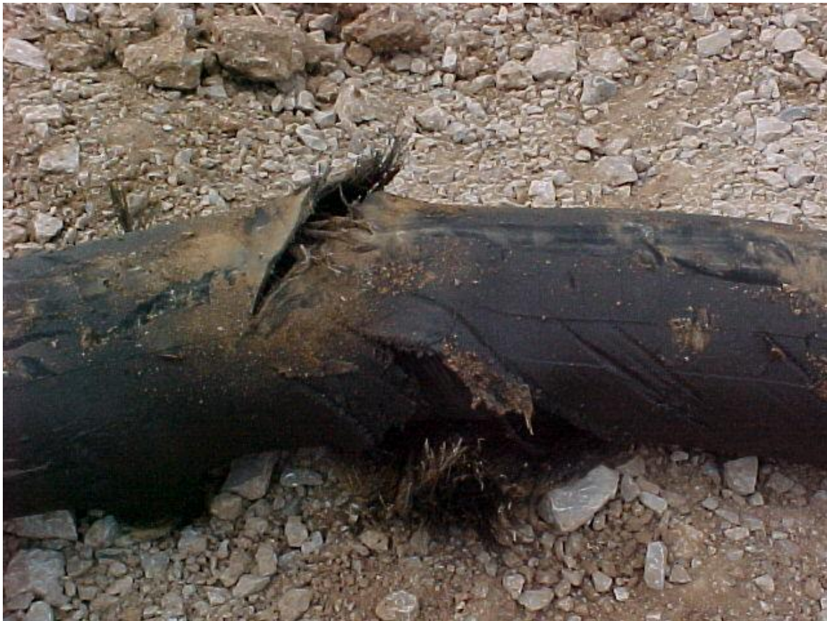
Figure 5.11 Corrosion induced failure, courtesy of Contitech
