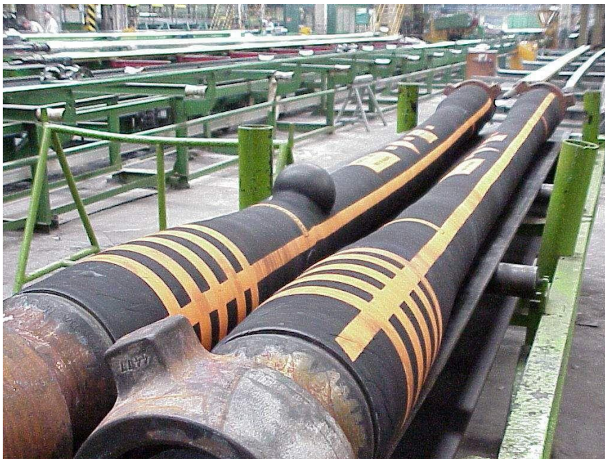
Figure 5.2 Pressure test with leaking liner, courtesy of Contitech
