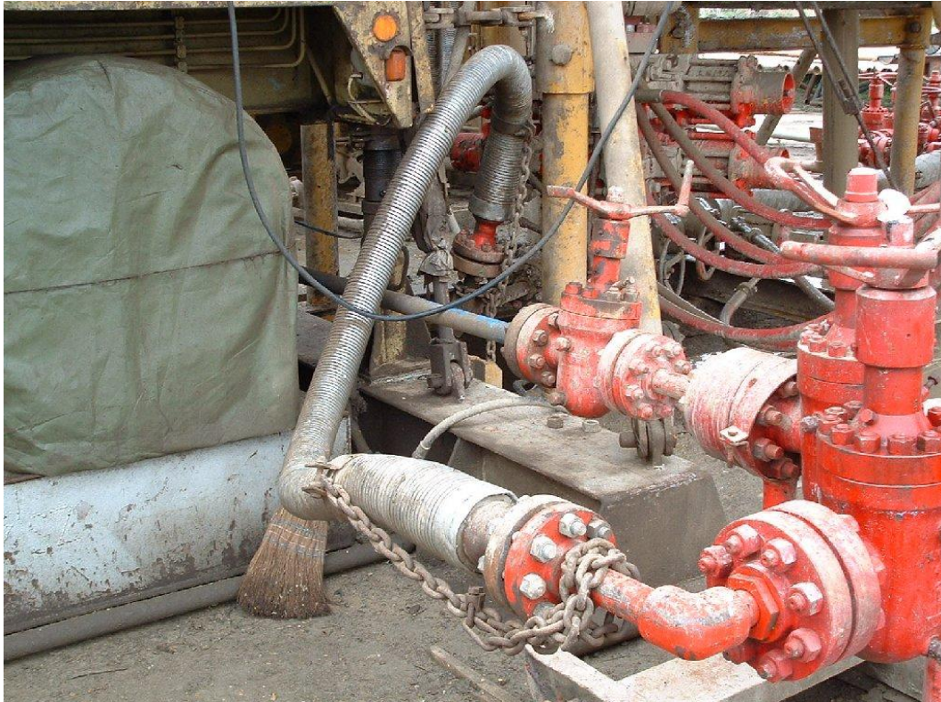
Figure 5.8 Over-bending example of bonded hose with external carcass, courtesy of Contitech
