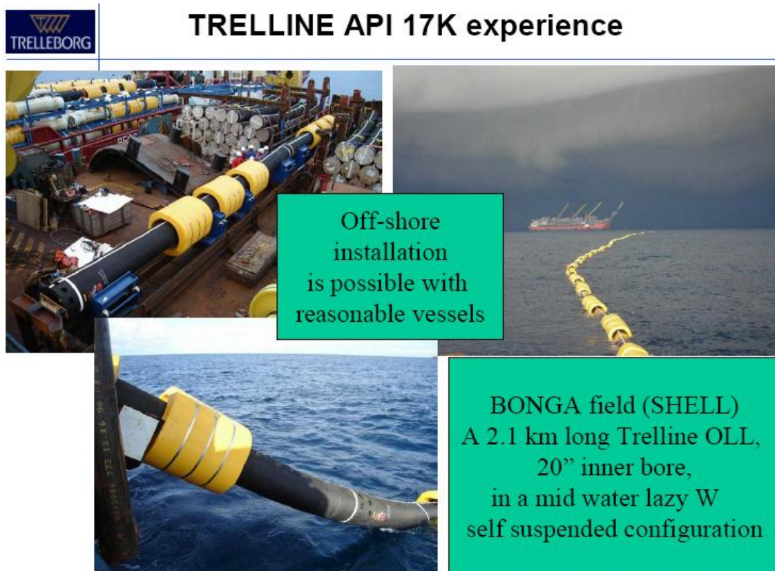
Figure 4.6 20" Trelline joints assembled to long length hose, courtesy Trelleborg
