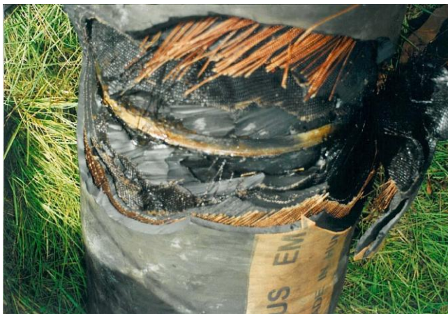
Figure 5.7 Excessive cover damage, courtesy of Contitech
