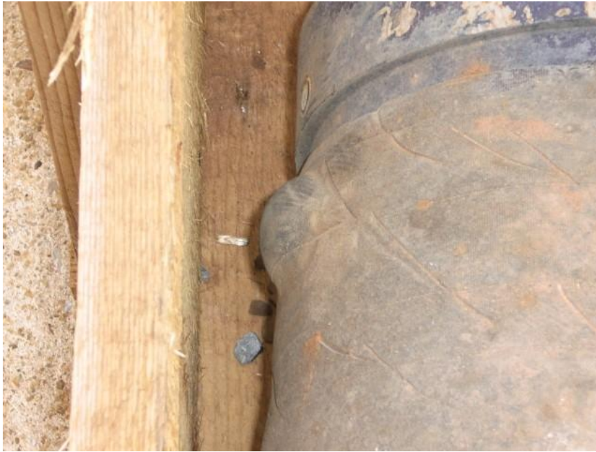
Figure 5.1 Bonding defect near end fitting detected in pressure test, courtesy of Contitech
