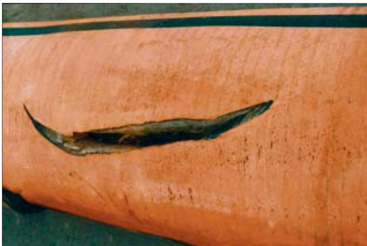
Figure 5.4 Propeller cut in floating hose (courtesy of Trelleborg)
