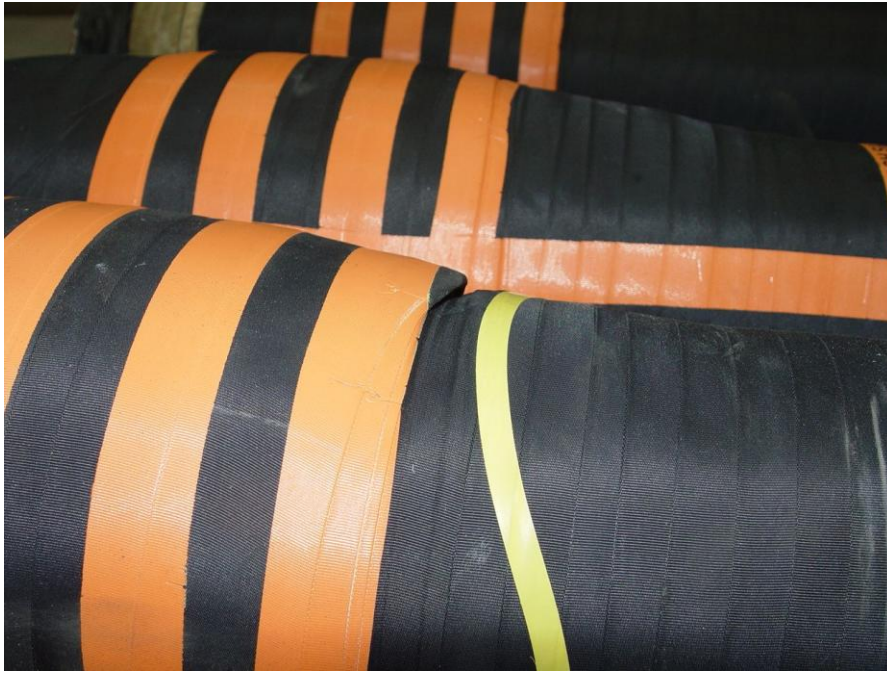
Figure 5.3 Cover damage example, courtesy of Contitech
