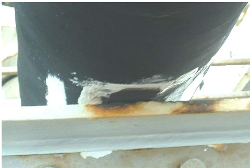
Figure 5.10 Abrasion and corrosion example, courtesy of Contitech
