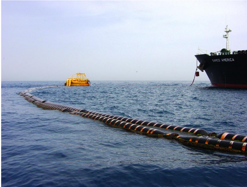
Figure 4.7 Floating hose, courtesy Dunlop Oil & Marine
