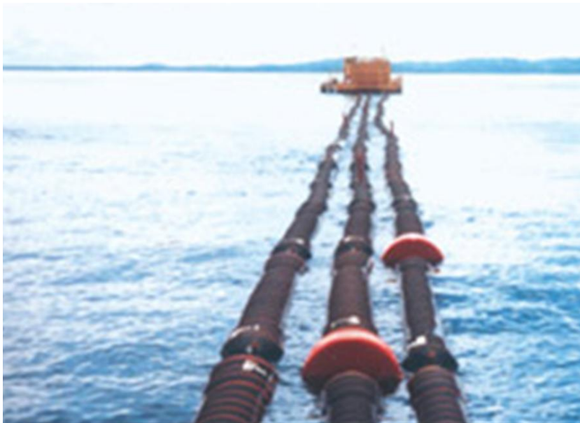
Figure 4.8 Double carcass floating hose, courtesy Manuli
