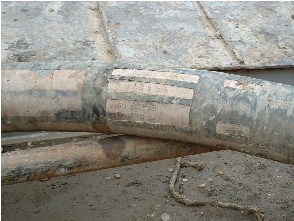
Figure 5.6 Old rotary hose, manufactured 1994, photo 2003 , courtesy of Contitech
