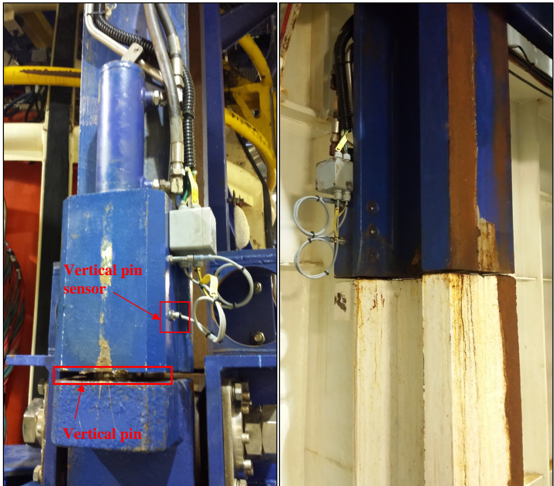
Figure 0-5: PICTURE 2 - Vertical locking pin sensor (left) and guiding rails (right)
