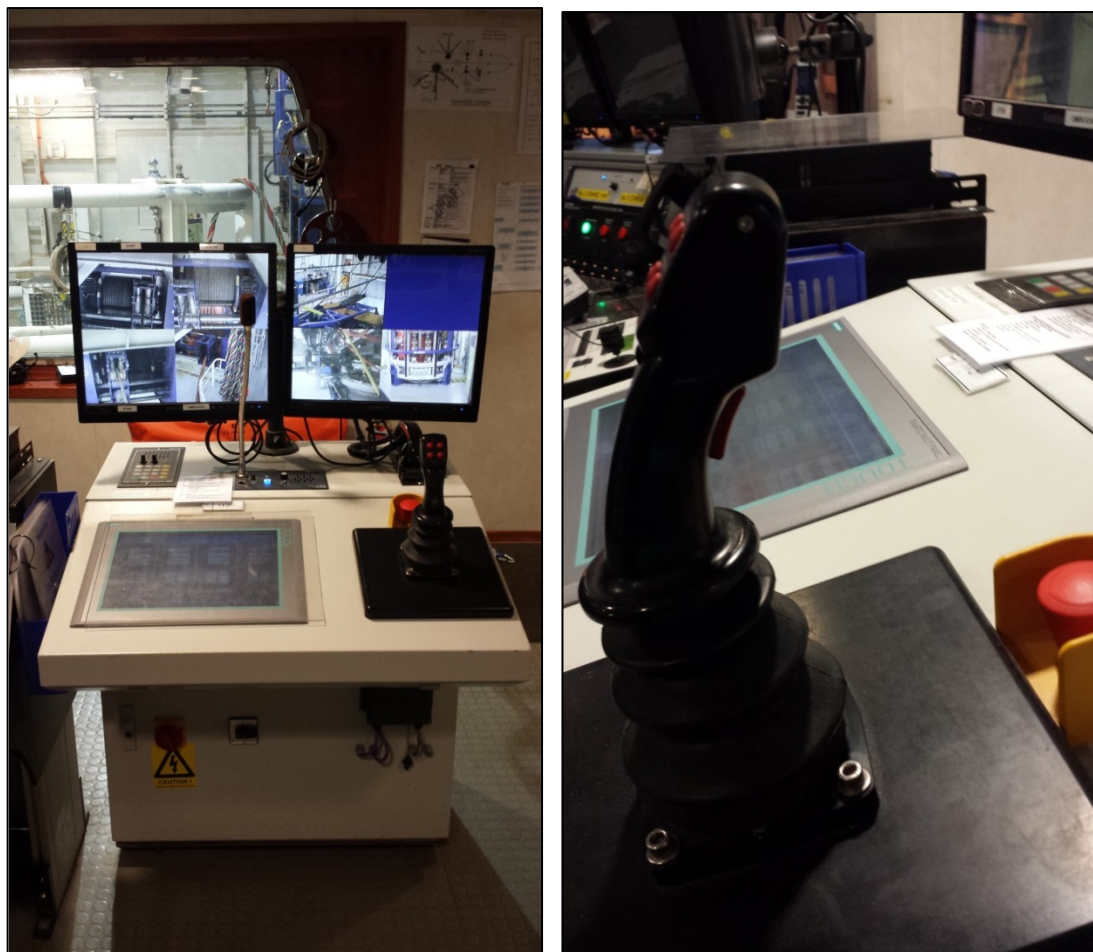
Figure 0-10: Port bell LARS station with cctv & HMI (left) and joystick with dead man trigger (right)
