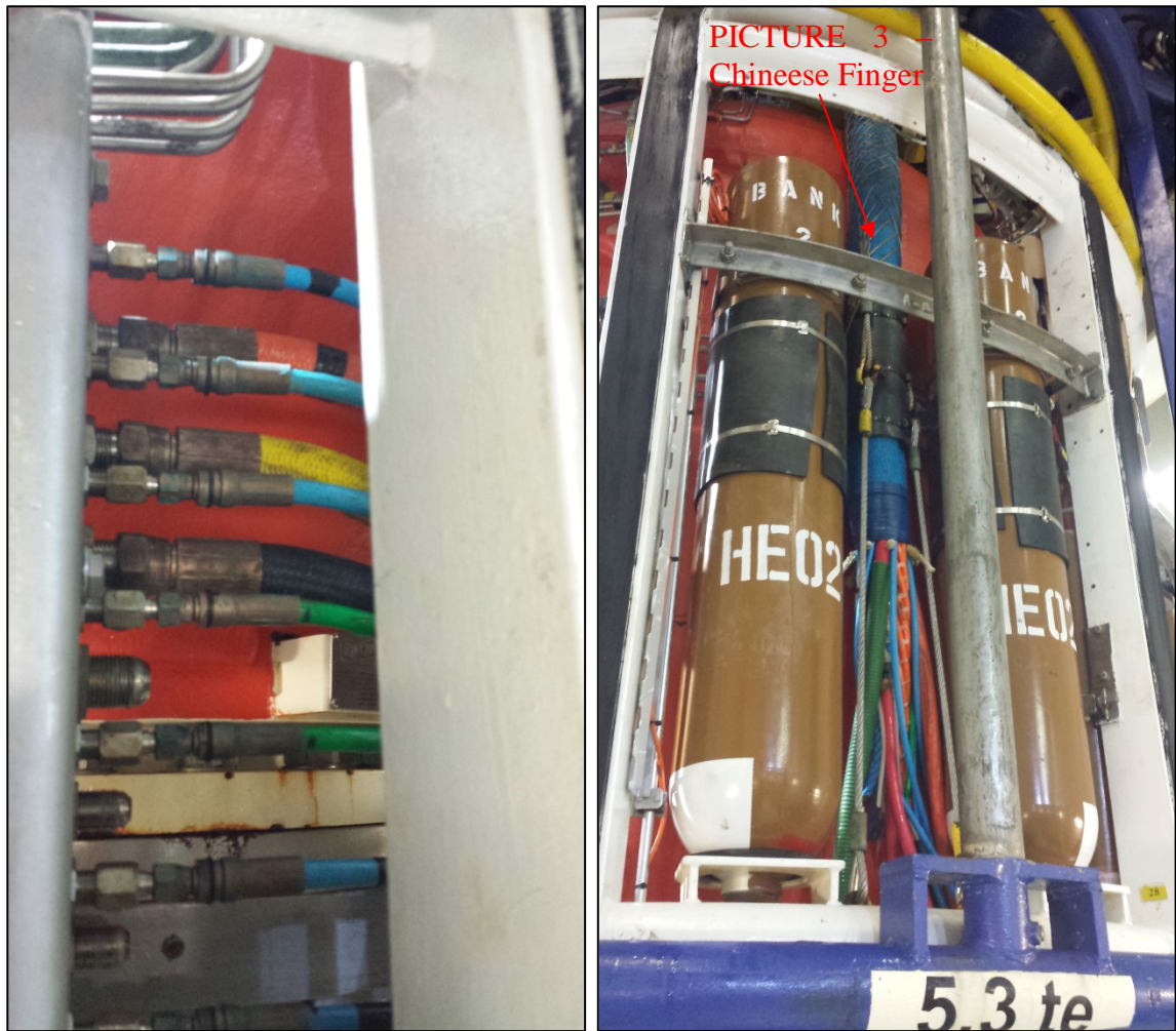
Figure 0-6: PICTURE 3 - Umbilical termination plate (left) and standard umbilical entry / termination (right)
