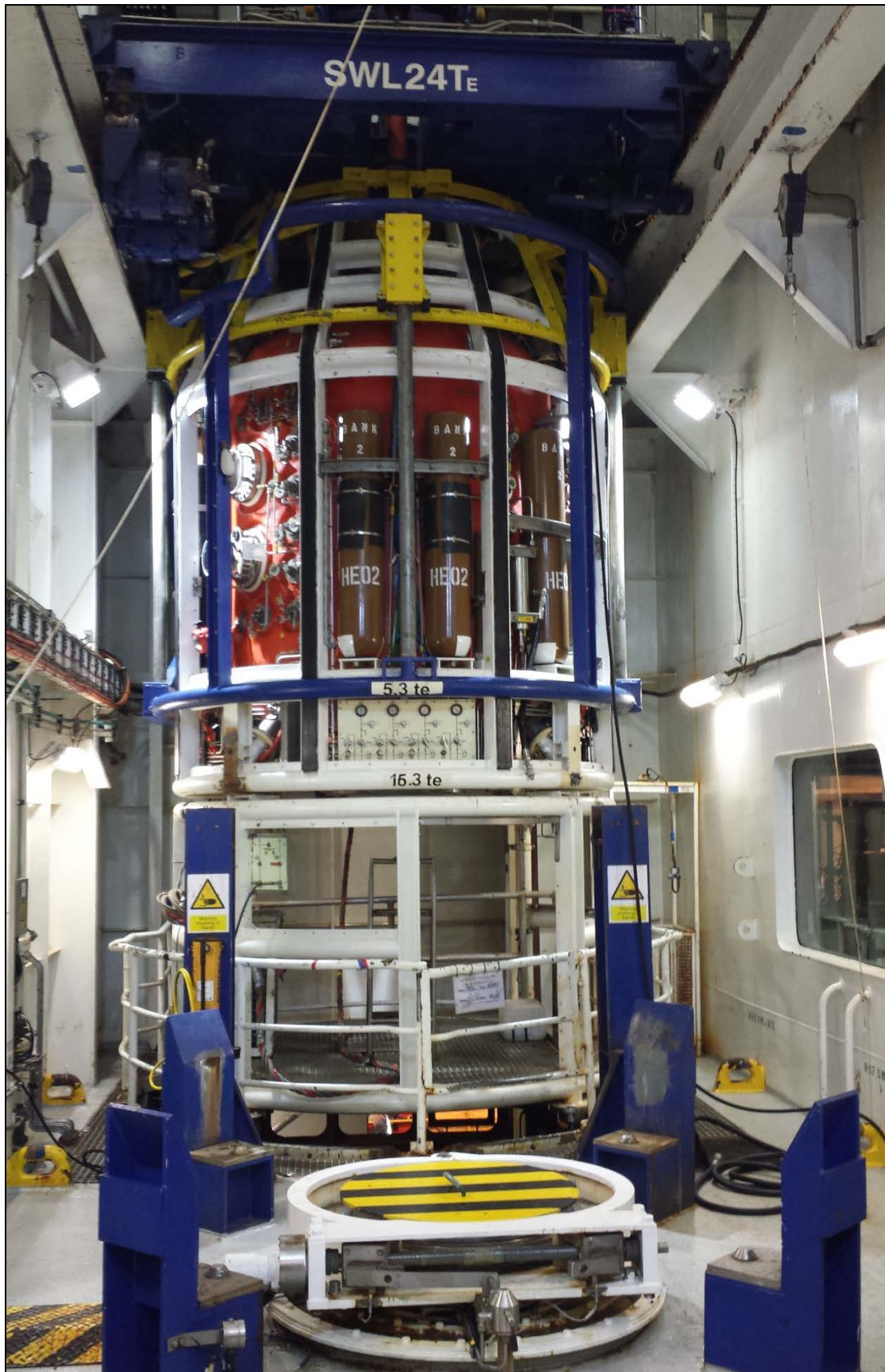
Figure 0-8: PICTURE 4 - Diving bell attached to stand off frame above deployment moonpool (stbd bell)
