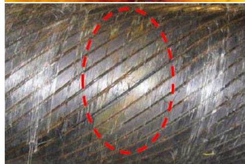
Figure 4-10 Typical external sheath cut with corrosion products on the surface, including wire inspection under the same damage, ref [28]
