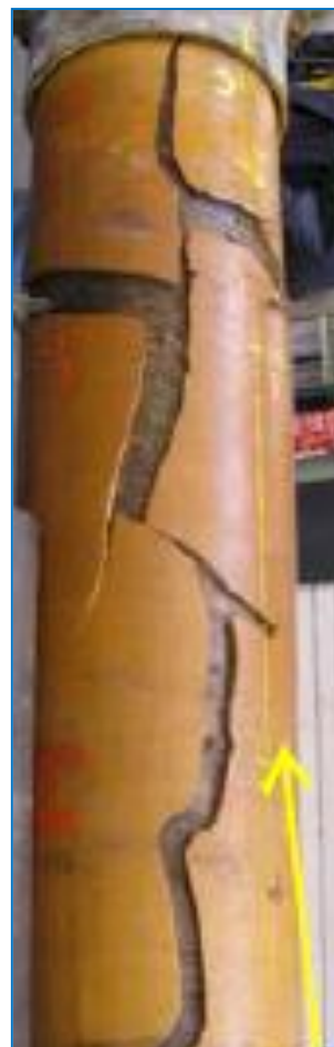
Figure 2-5 External sheath cracking due to high temperature under bending stiffener, ref [14]
