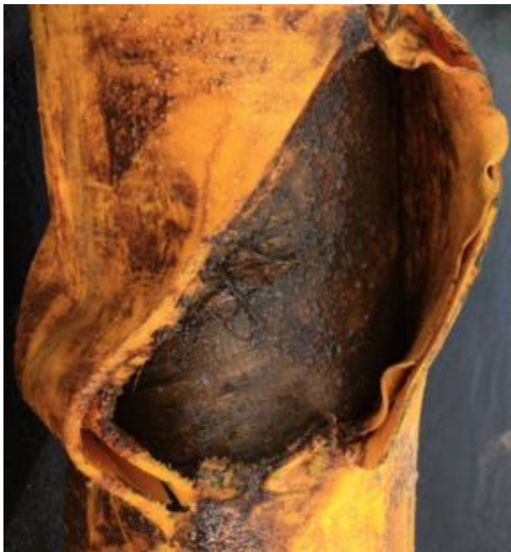
Figure 1-3 Typical external sheath failure due to pressure increase in the annulus, double external sheath (4subsea)
