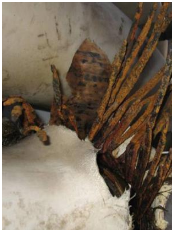
Figure 3-7 Severe corrosion lead to flexible pipe failure in Norway, however not reported as this is not a riser suspended overboard
