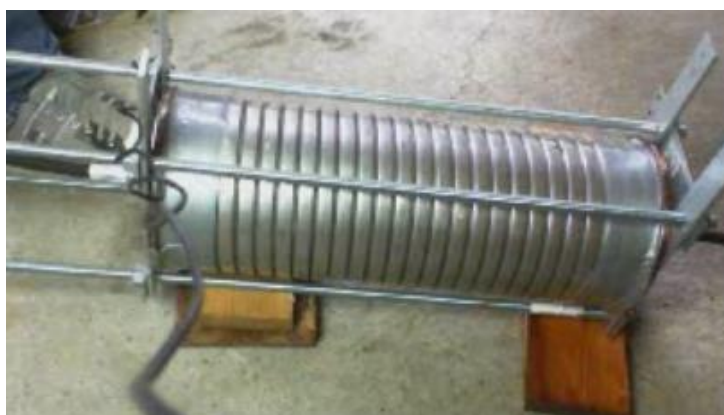
Figure 4-12 Testing of carcass radial leak rate (4Subsea)
