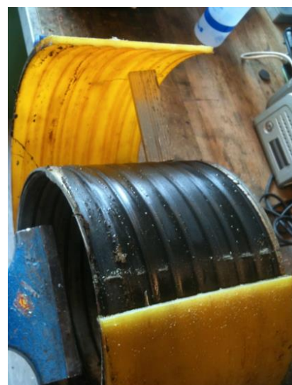
Figure 5-2 PA11 coupon extracted for analysis (Statoil), ref [28]
