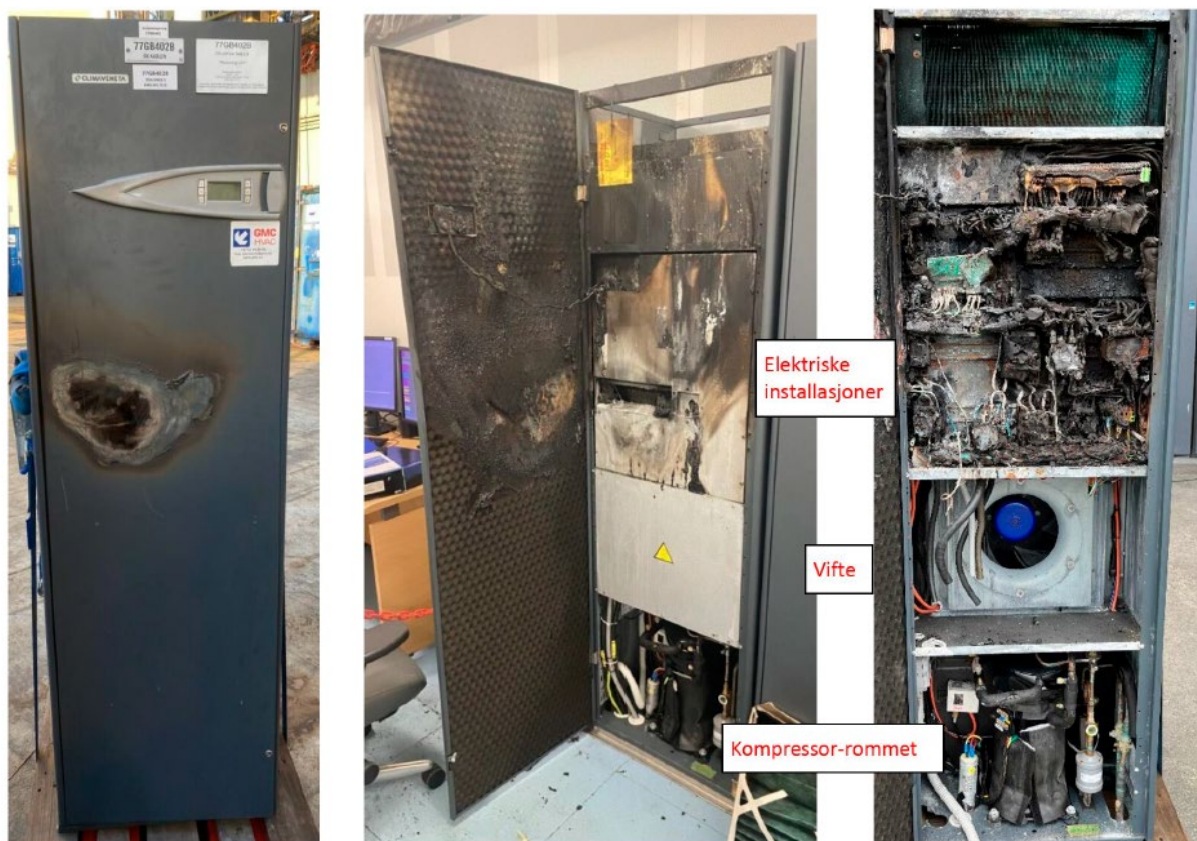
Figure 5 Cooling unit with cabinet door closed (left), open (middle), and after three internal panels/covers were removed (right). (Source: SINTEF Report 2023-01109 Fire in DX unit on the Gina Krog - Rev 1.0 (part 1))
