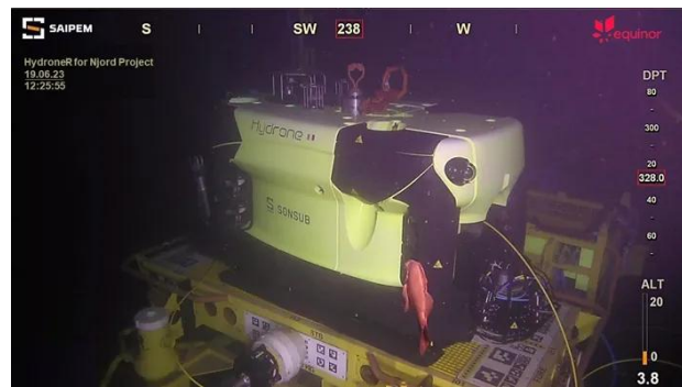
(b) Saipem's Hydrone-R with Subsea Docking Station by BlueLogic 13, 14 .
