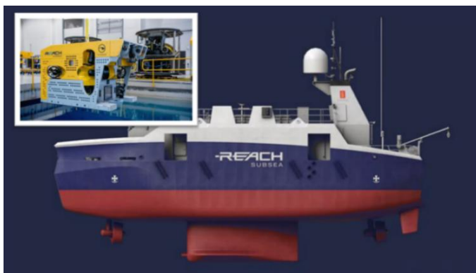
Figure 4.4: Reach Subsea and partners have developed a USV, which is used to launch ROVs. The picture is reproduced with permission by Reach Subsea.
