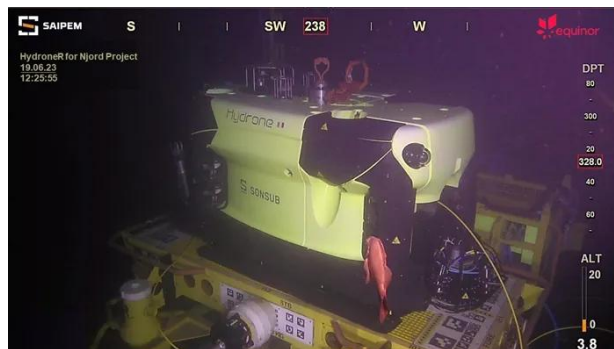
(b) Saipem's Hydroner-R med Subsea Docking Station (SDS) fra BlueLogic 13, 14 .
