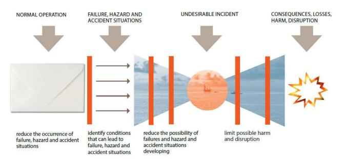
Figure 2 Barrier diagram showing how barriers, in red, are used in to reduce risk
