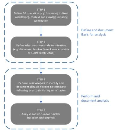
Figure 8 Methodology for Estimating Time to Safely Terminate DP Operation
