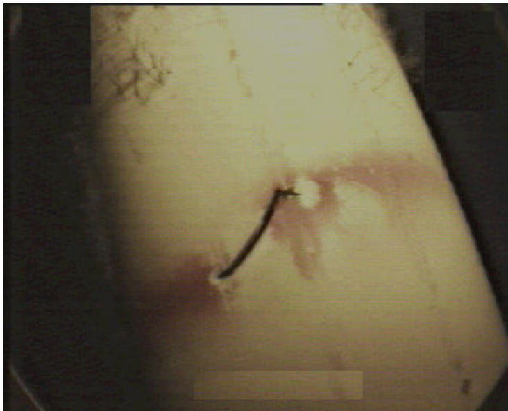
Figure 3-6: Armour wire corrosion due to external sheath damage (Statoil)
