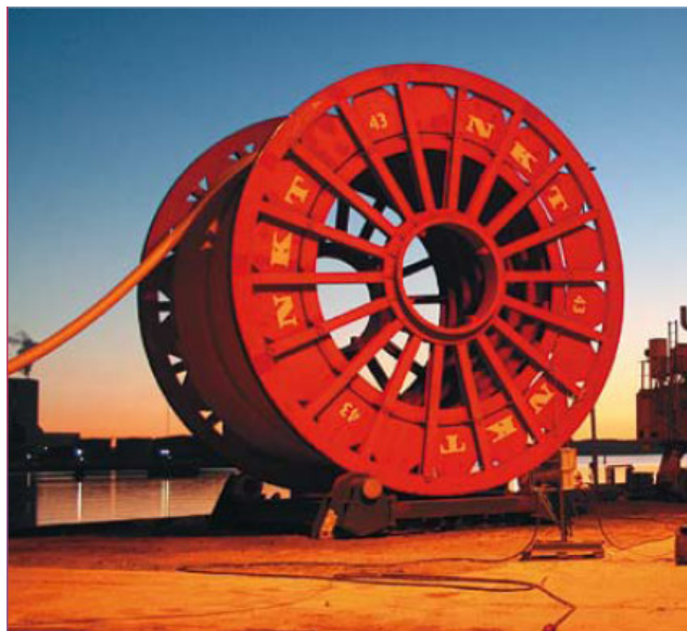
Figure 3-4: Flexible pipe transportation / installation reel (NKT)
