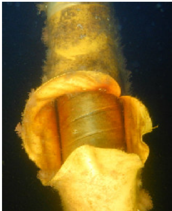
Figure 3-8: Burst external sheath due to blocked vent system.
