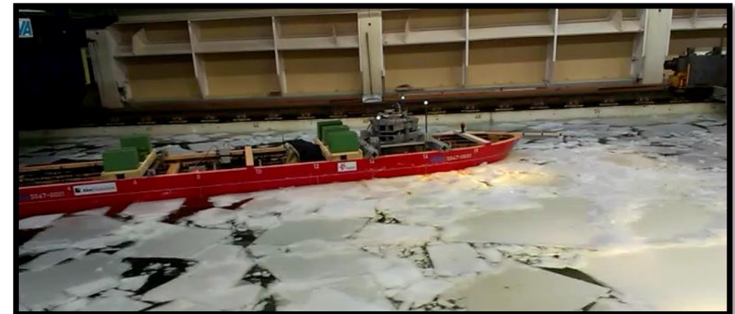
April 2013: Ice tank tests of the Johan Castberg hull
