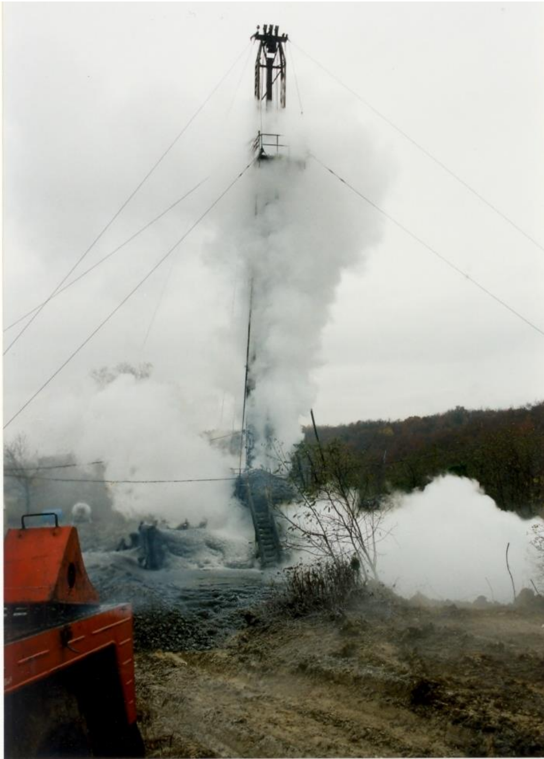
Figure 3 - CO 2 Blowout Case History – Vapor cloud visibility, freezing CO 2 temperatures [Courtesy of Wild Well Control]
