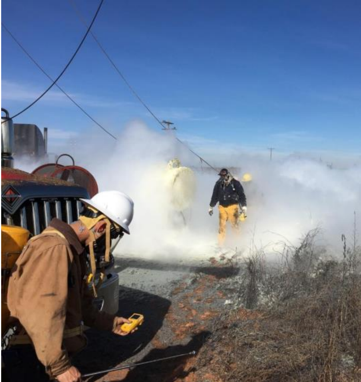
Figure 2 - CO 2 Blowout Case History – Blowout Location Ingress/Egress under SCBA Visibility cloud [Courtesy of Wild Well Control]
