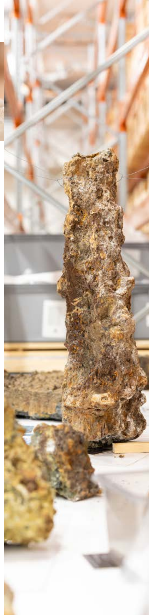
Inactive sulphide chimney on the seabed: Seawater has first penetrated into the subsurface, been warmed and taken minerals with it. When the water flowed back up and hit the cold ocean water, this chimney-like sulphide structure was formed.
