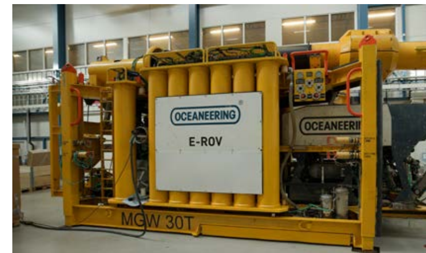
Liberty is an autonomous subsea platform that provides power, communication and support to underwater vehicles on the seabed.
