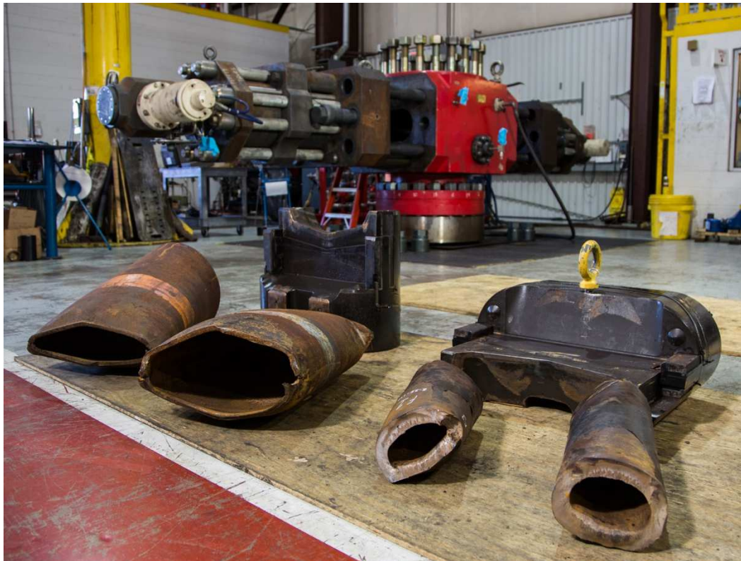
Figure 11 Chevron's dual ram Alternative Well Kill System, AWKS (Courtesy of Chevron)
