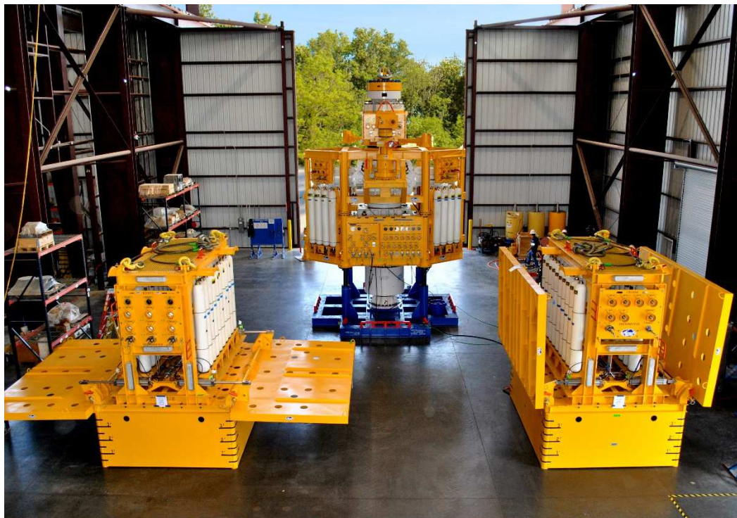
Figure 10 Trendsetter Arctic Class 18 ¾" 15,000 psi drill through Mudline Closure System (Courtesy of Trendsetter Engineering)
