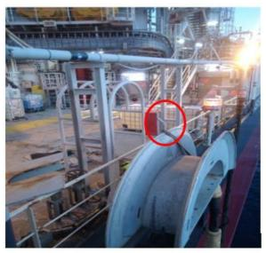
Figure 4.4 Port saddle and protector. The bracket with safety strap is illustrated by a red circle (photo: police).
