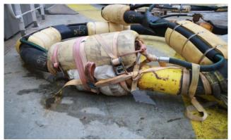
Figure 4.10 Valve block and flange with extra protection (photo: police)
