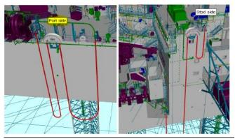
Figure 4.1 Free-hanging cuttings hoses, port and starboard sides (source: KCA Deutag).
