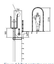
*Figure 4.2 Port protector on construction drawing AfC 24 March 2016, revision 5 (source: Samsung/Statoil).*
