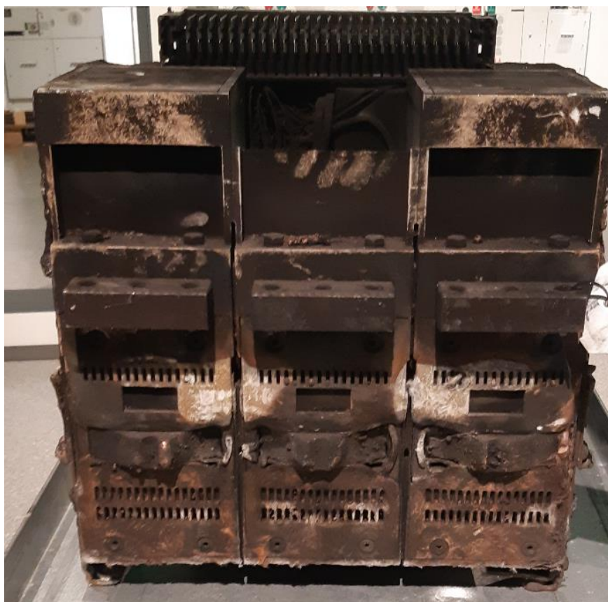
Figure 8 Damage to the lower contact set on the spare breaker.
