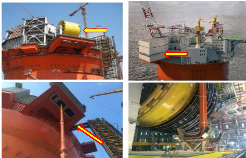
Photograph 2: Top left: offloading hose before enclosure. Top right: D10 area in front of the flare boom after enclosure. Above left: offloading hose seen from the sea. Above right: the reel with the loading hose viewed inside the D10 area. (Source: Eni)
