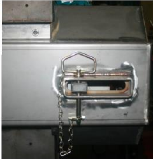
Figure 9: Photos from the NOV safety report show the correct installation of the safety pin.
