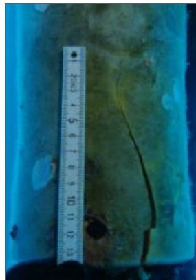
Stiffener Tip Damage
