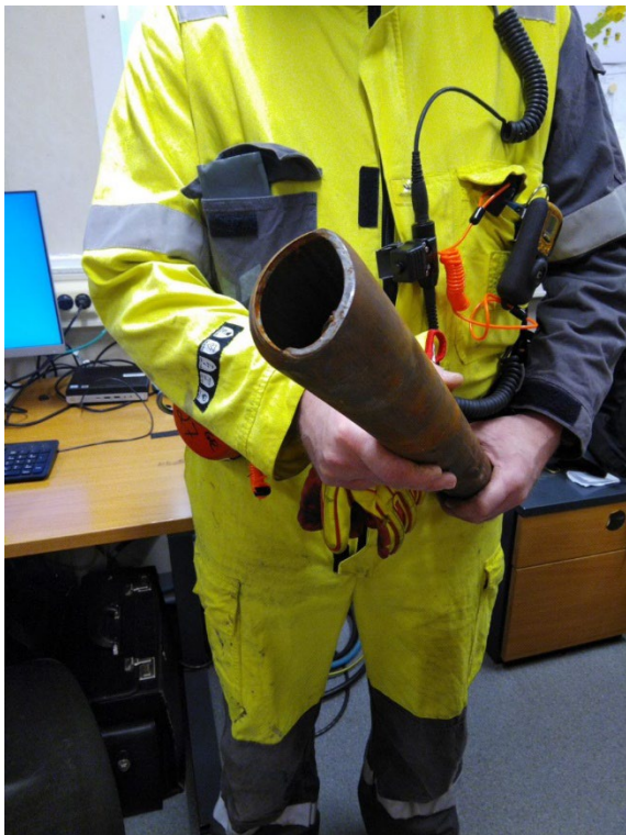
Image 4 - Tube stump after being cut by the CT BOP.
