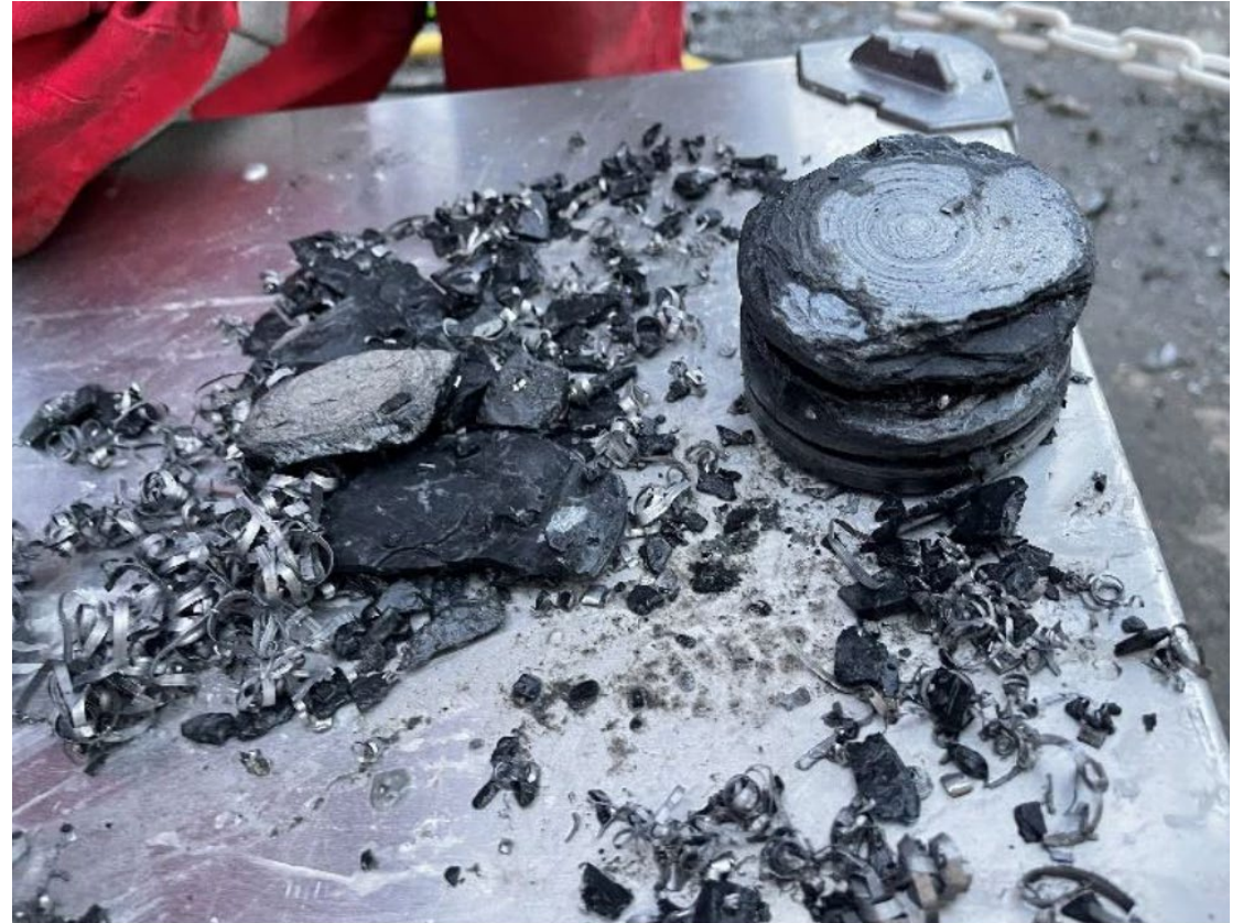
Figure 16 - Delaminated section of grout from core 3 from Elev. 3.91m.
