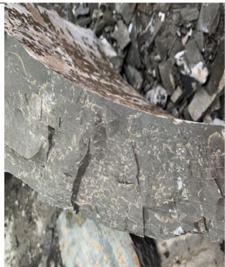
Figure 30 Layering/hairline cracks in the grout body, seemingly calcified circumferential cracking in the grout volume.
