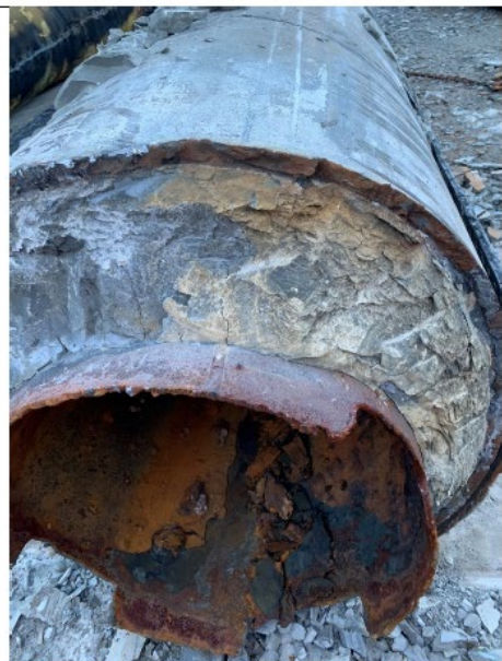
Figure 28 Pile Sleeve connection prior to splitting. Some intrusions
