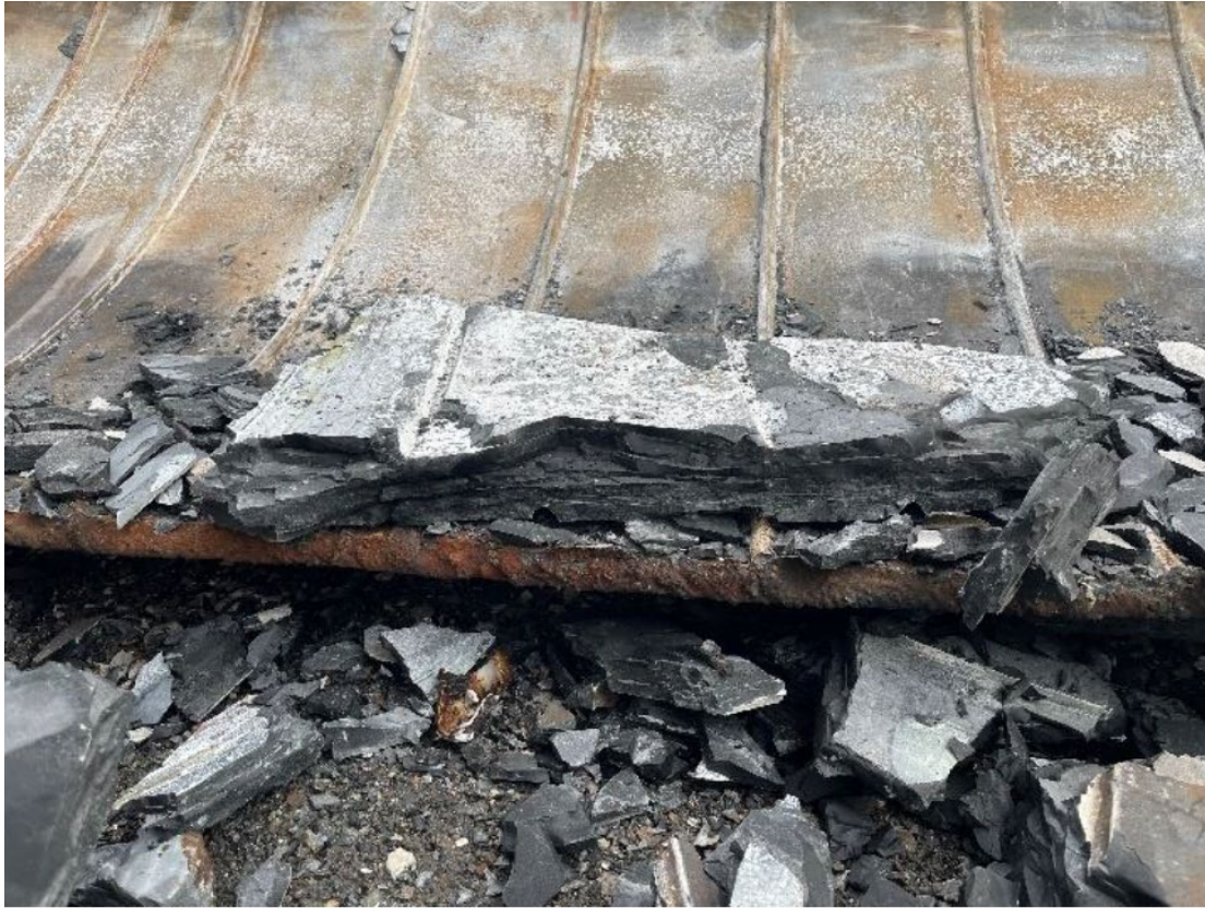
Figure 5 - Layering of grout material at approx. 4m elevation from bottom of connection
