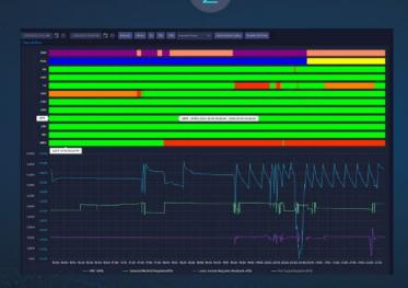
A significant increase in pump input was identified with an interval of 10-11 minutes
