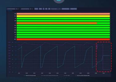
After the request, the RTOC contacted Subsea, and they began troubleshooting together to identify the issue. Around 7 PM (Houston Time), after placing the Stack Mounted Accumulators in Block, the Accumulator Trend returned to a more stable pattern
