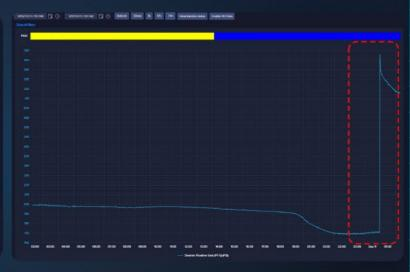
Open Under Differential Pressure was detected when the Middle Pipe Ram was opened
