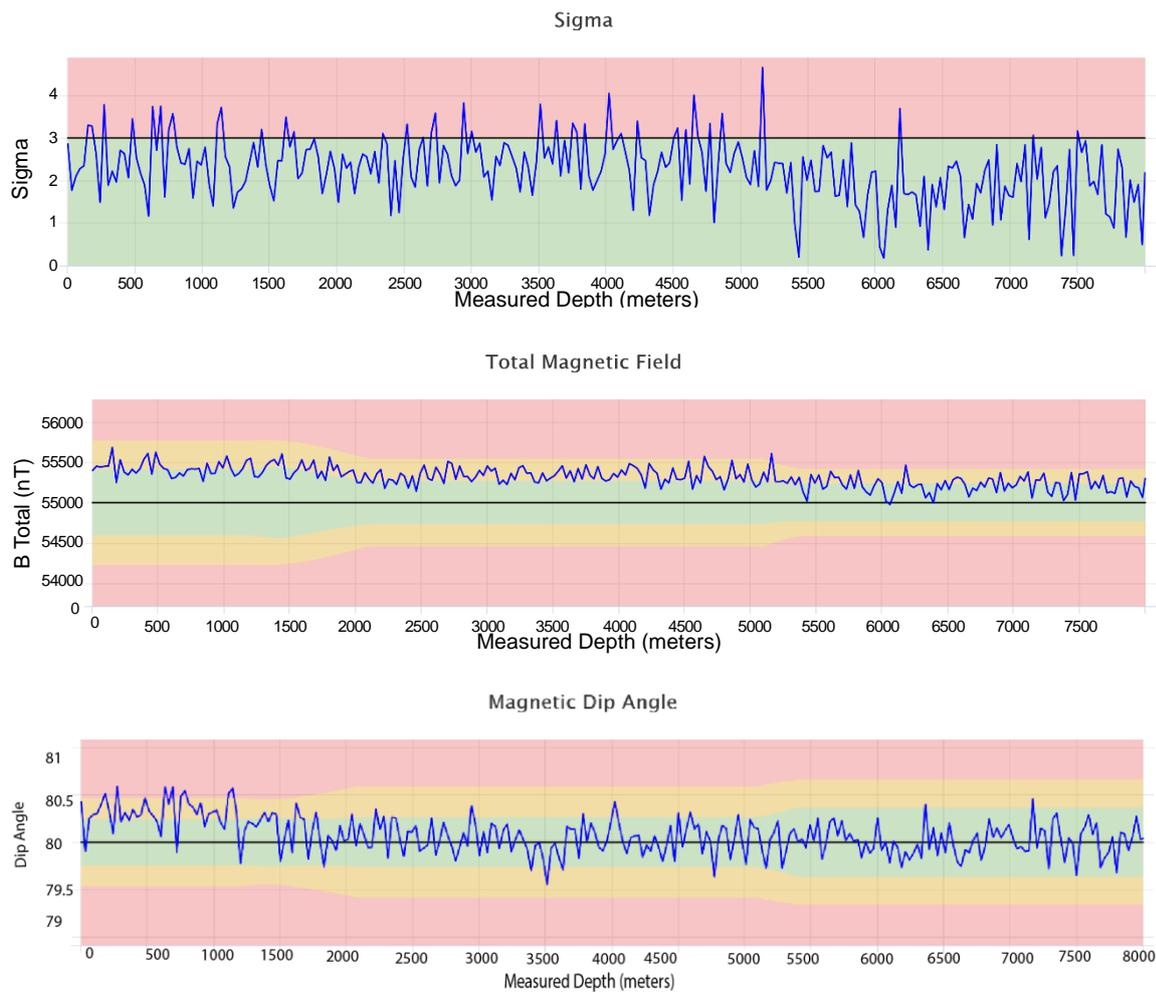
Figure 5.7: Well #3 simulated quality control values for drilling at a 45 degree azimuth with standard referencing
