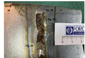
Magnified area with corroded weld.
