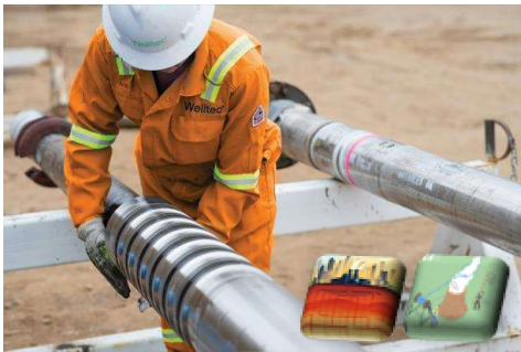
Field Engineer preparing metal expandable packer for deployment, USA land operations.
