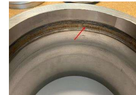
Magnified area Piece 1: 8,5" component. After the test. Only light orange corrosion products.
