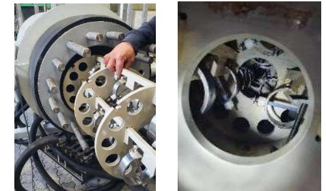
Placement of the material coupons inside the test chamber (30 coupons in total)
