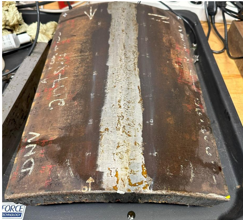
Figure 7 – The test object containing HACC.
