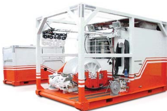
Figur 8-23 Wireline skid (ref. NOV)
