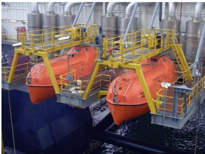
Figur 10-7 Norsafe livbåt med utligger davit A-110 MKI (ref. http://norsafe.com/lifesavingsystems/davits/conventional-davits/a-lifeboat-davit-series/ )
