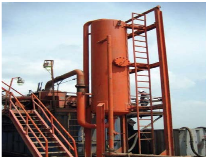
Figur 8-11 Mud / gas separator (ref. DC Mud systems)
