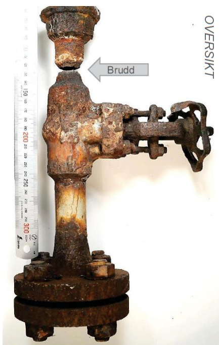
Figure 7: Configuration of the branch pipe with the end to the main pipe on top, the packing box valve and the blind flange. The arrow points to the fracture site. Scale in millimetres.
