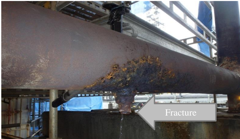
Figure 6: Main pipe with pipe end where the fracture occurred. The pipe end was later removed for material technology investigations. The scale of external CUI can be seen.
