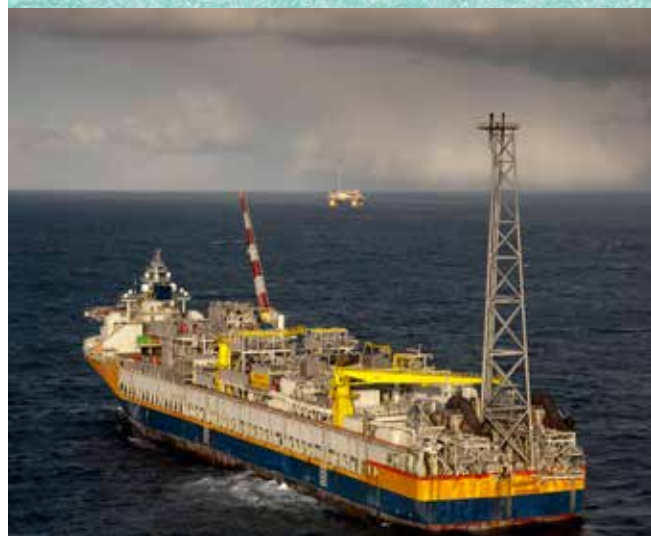
The Åsgard A production and storage ship is one of three floating facilities on this Norwegian Sea field. More than 50 subsea wells have been drilled down on the seabed. (Photo: Øyvind Hagen/Equinor)
