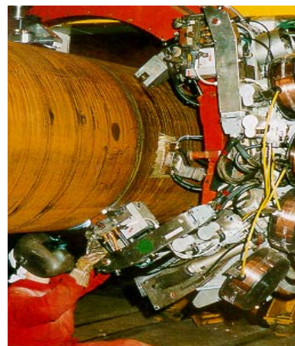
Figure 4. Saturnax welding system (LB 200), and detail of welding heads.
