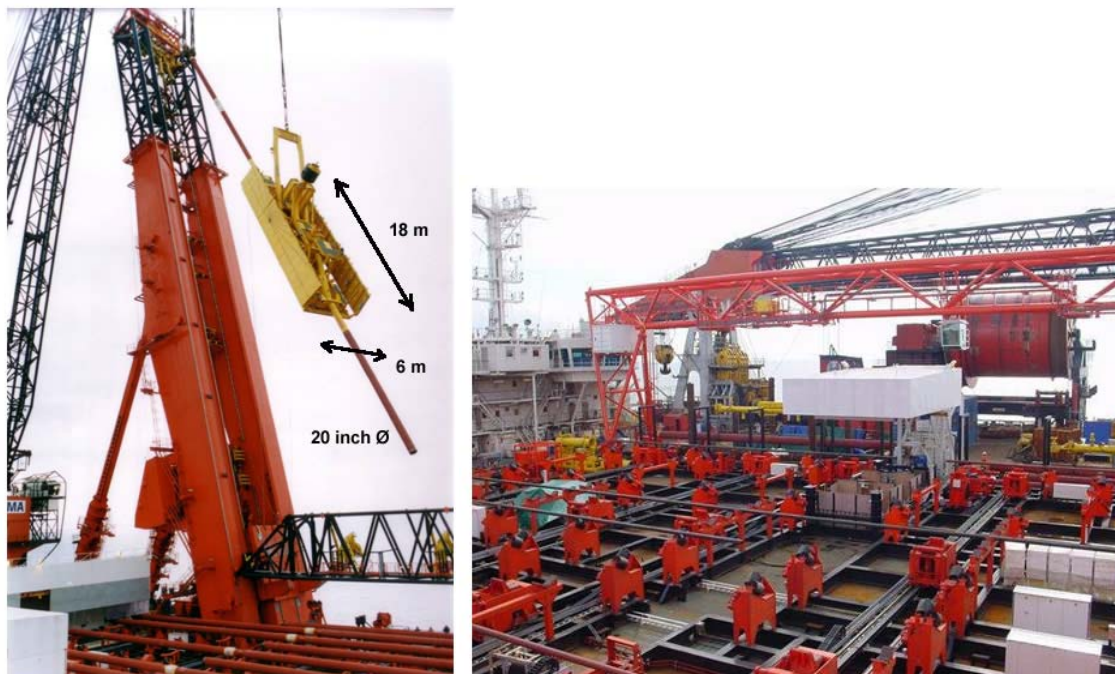
Figure 5. "Balder: a) Pipeline tower and b) deck area arrangement for pipe-laying (photos courtesy of Heerema Group).
