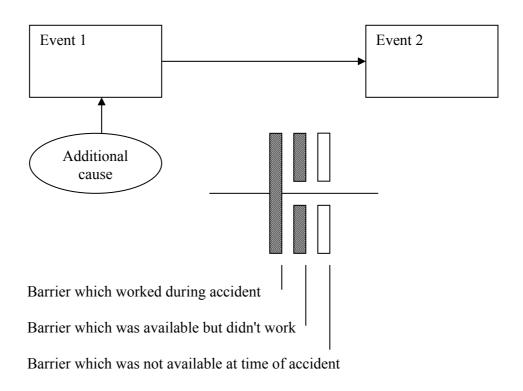
Figure 1:Sample barrier diagram.
