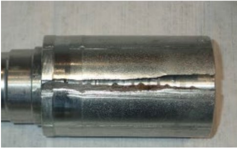
Photo 7: Sleeve with an axial fracture (Source: Equinor)
