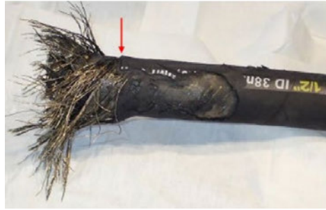
Photo 8: Torn hose end (Source: Equinor)
