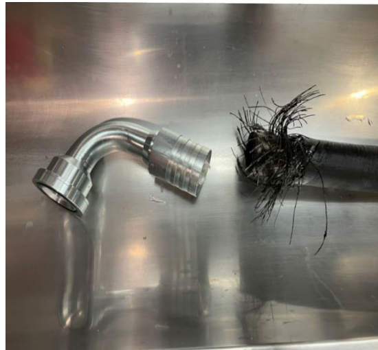
Photo 10: Press coupling with the end of the hydraulic hose (Source: Equinor/Island Offshore)
