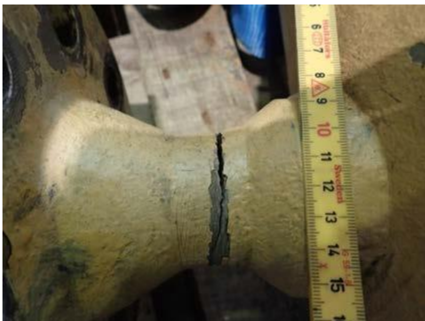
Figure 4: The rupture (photograph from Statoil's material technology investigation).
