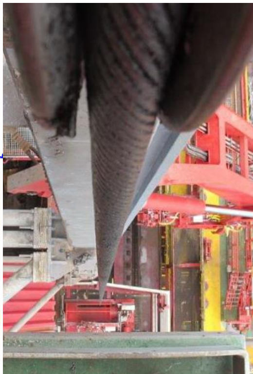
Figure 6: The fleet angle between drum and sheave.
