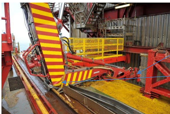
Figure 10 The crane with bent crane arm and broken gripper arrangement.
