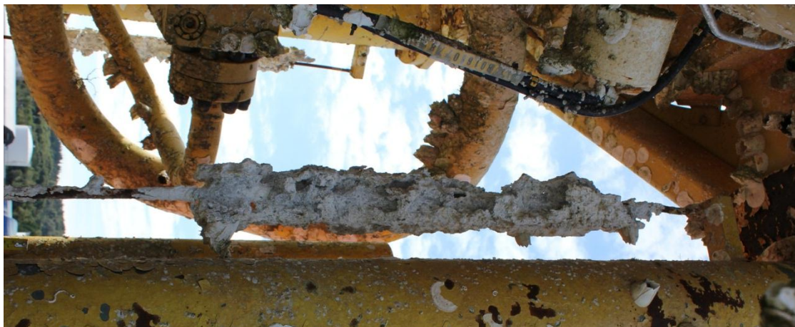
Figure 7.2 Example on totally consumed galvanic anode
