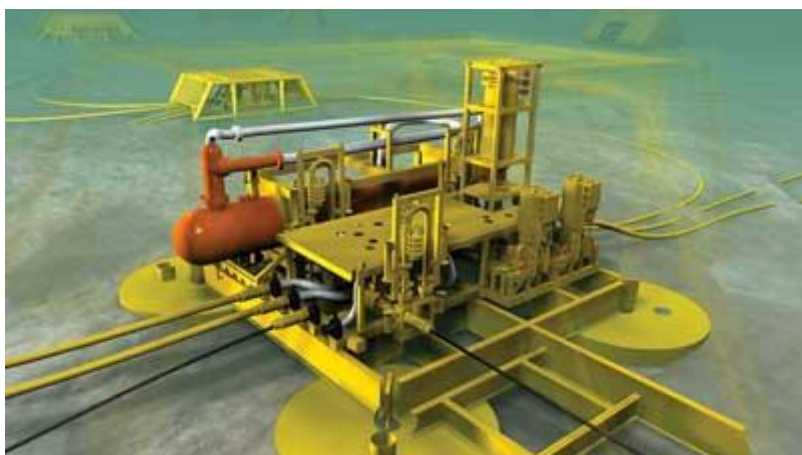
Figure 3.10 Tordis - the world's first full-scale, commercial subsea separation, boosting and injection system
