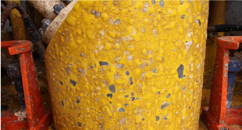
Figure 7.1 Example of coating breakdown after approx. 15 years in service.
