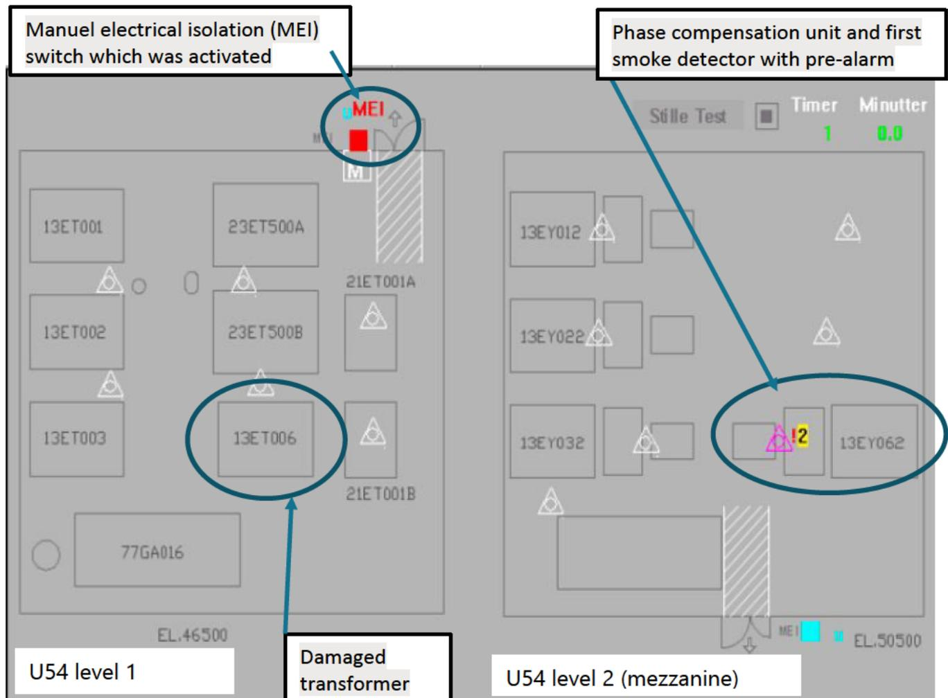
Figure 7: High-voltage transformer room U54, levels 1 and 2. Source: Equinor
