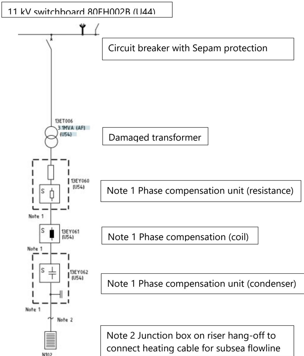
Figure 9: Extract from single-line diagram for the DEH system.
