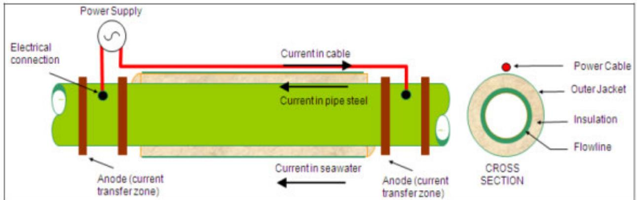
Figure 8: Direct electric heating (DEH) system – open loop (wet insulated)
