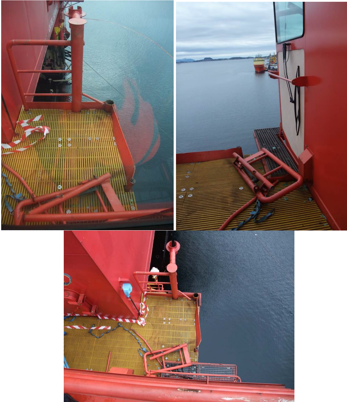
Figure 43: The area by the operating house where the pennant wire destroyed its holder, the railings and the operating house window. The damaged window is covered here with a wooden sheet. The holder for pennant wire 7 remains. The photographs were taken in Kristiansund in November 2012 by the PSA.
