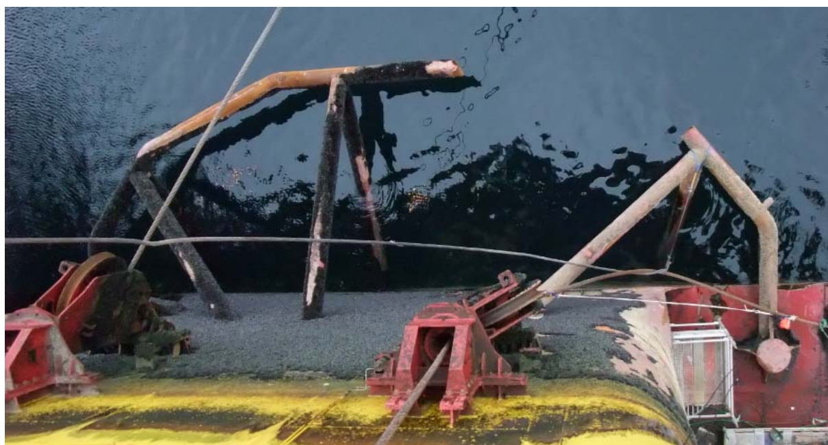
Figure 12: The bolster after the damage. Line 7 is to the left and line 8 on the right. Line 7 has been used here for mooring to land. The line running across the picture is the pennant wire. A comparison with Figure 11 shows which components have fallen off. The photograph was taken in Kristiansund on 13 November 2012 by the PSA.
