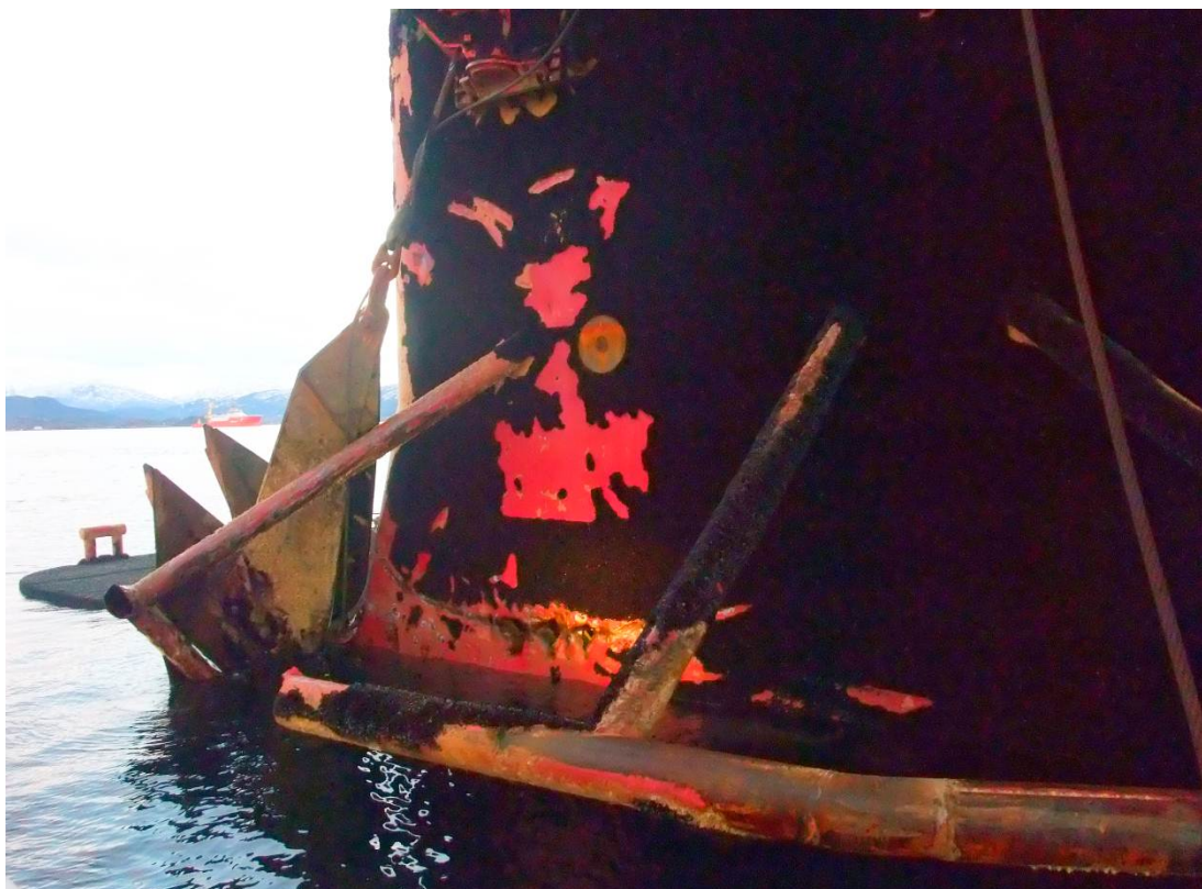
Figure 3: Anchor 8 and the damage above the waterline, here at transit draft. The anchor which caused the damage and the partly destroyed bolster are visible. The photograph was taken by the PSA on 10 November 2012 in Kristiansund.
