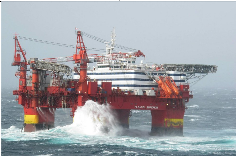
Figure 1: Floatel Superior at survival draft (13 metres). The air gap is 14.5 metres from sea level to the underside of the topside (beneath the text “FLOATEL SUPERIOR” in the photograph). Spray from the wave in the foreground reaches the drum of winch 4 (with anchor line 8) on the forward port column. The photograph was taken during an earlier episode of bad weather. Copyright Erik Sevaldsen 1 .
