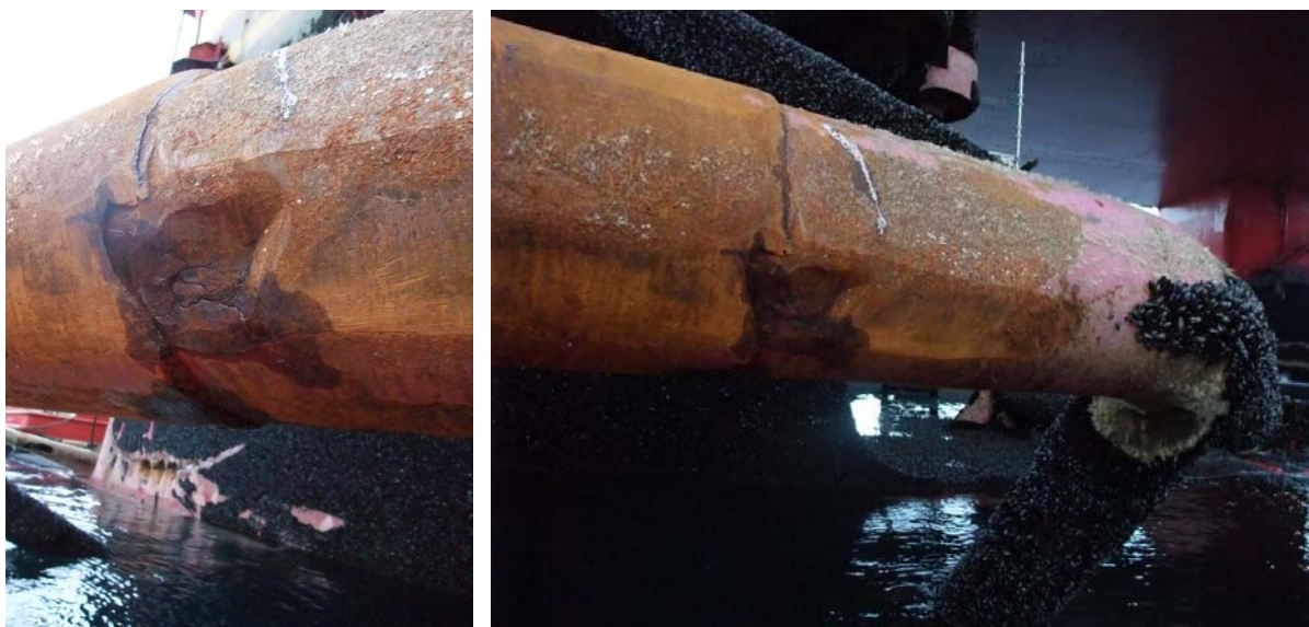
Figure 30: Wear damage where anchor 7 has been wrongly positioned on the bolster (towards the aft of Floatel Superior ) and worn bolster material and wear surfacing on the edge of the wear surface (left). Note also the surface which has been scraped smooth on the bolster base material to the right. These observations are interpreted to mean that anchor 7 (and other anchors similarly) moved for long periods outside the dedicated position on the bolster's wear surface. In addition, the local wear on the edge of the wear surface is interpreted to show that the anchor has been "locked" in this position and that a high contact pressure has led to extensive local wear. With movements of the anchor from the centre of the wear surface, the geometry of the bolsters causes the wire rope to elongate. This design is intended to
