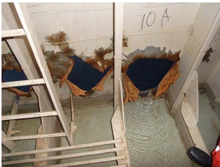
Figure 4: Three of holes in tank 10A viewed from inside. The photograph was taken in Kristiansund during November 2012 by the PSA.
