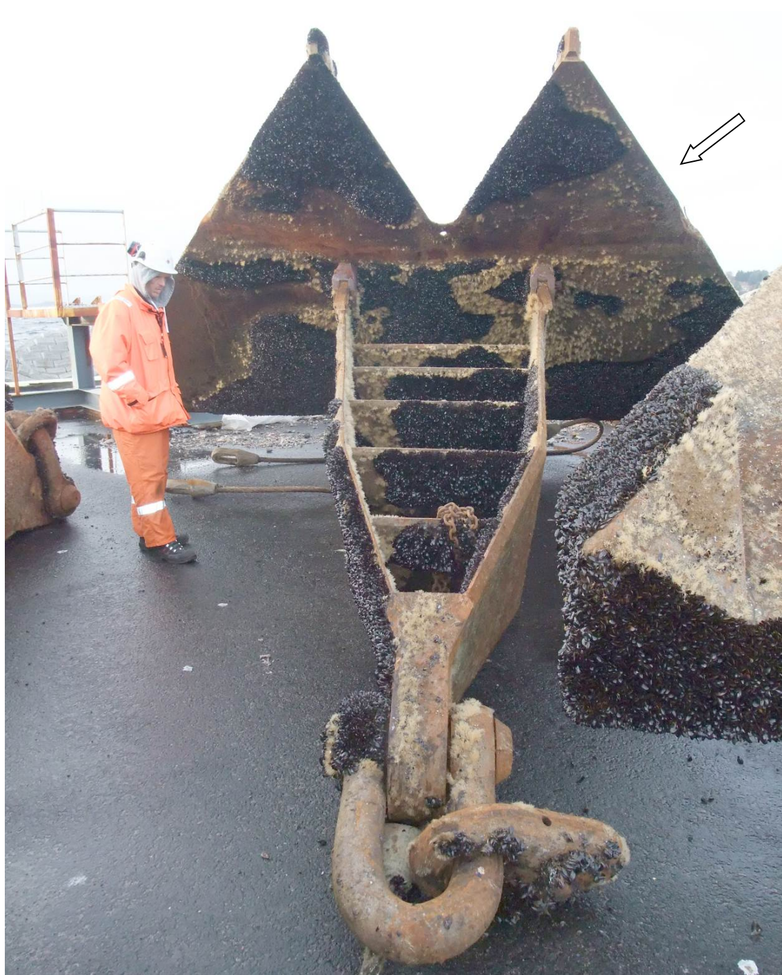
Figure 2: A 12-tonne Bruce anchor from Floatel Superior . The photograph shows anchor 1 from the starboard side after removal. The scratch marks where marine fouling (the blue-black colour of the mussels) has been removed show that the anchor has rotated as well as moved from side to side (see the fan shape on the right-hand side of the fluke, arrowed). See also Figure 14, which shows various positions taken by the anchor. The anchor fluke is the large plate topped by two points. The photograph was taken by the PSA on 14 November 2012 in Kristiansund.
