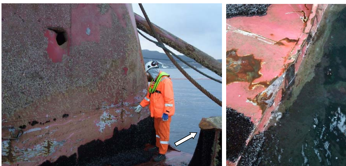
Figure 13: The hull at the front of the column outside tank 10. A simple penetration before the anchor has become wedged between hull and bolster components. Note the bent plate marked with an arrow in the left-hand picture. The picture to the right shows extensive wear on hull plates outside tank 2. The photographs have been taken by the PSA in Kristiansund on 12 November 2012.
