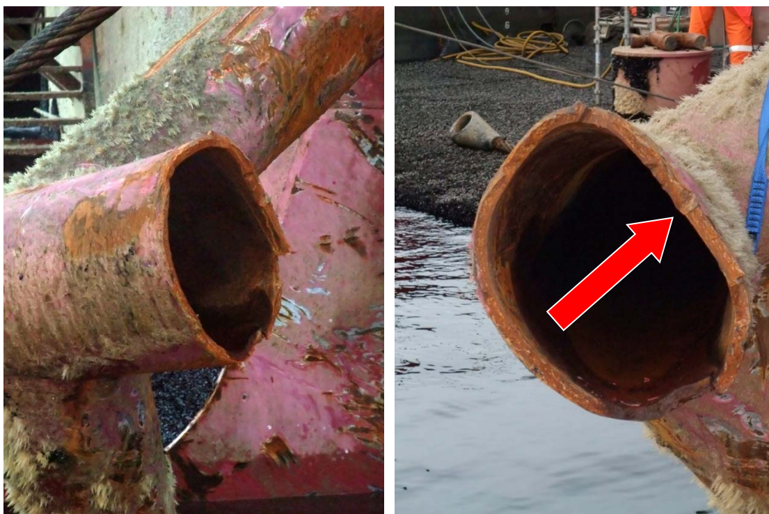
Figure 31: Fracture surface B on the bolster, see Figure 27. The fracture has developed from the circumferential weld at the bend in the bolster geometry. Note that the final stage of the fracture could have developed as a tension fracture from the anchor tension (along the arrow), and the cross section has been deformed to a straight section before this component was torn off and the A-B bolster section fell off shortly before 01.40. The photographs were taken in Kristiansund on 12 November 2012 by the PSA.
