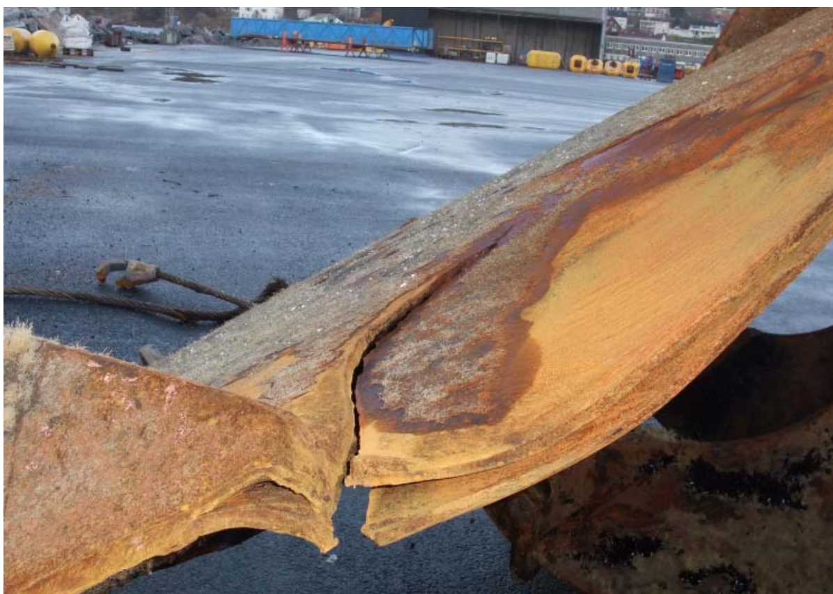
Figure 10: Damage to anchor 8 on Floatel Superior , photographed in Kristiansund on 14 November 2012 by the PSA.
