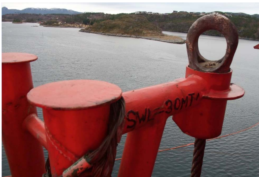
Figure 15: An intact pennant-wire holder on Floatel Superior . The wire is freed by lifting the loop away from the hull with a crane. The whole steel structure for wire 8 was ripped off, including holder and railing. The photograph was taken by the PSA in Kristiansund on 13 November 2012.
