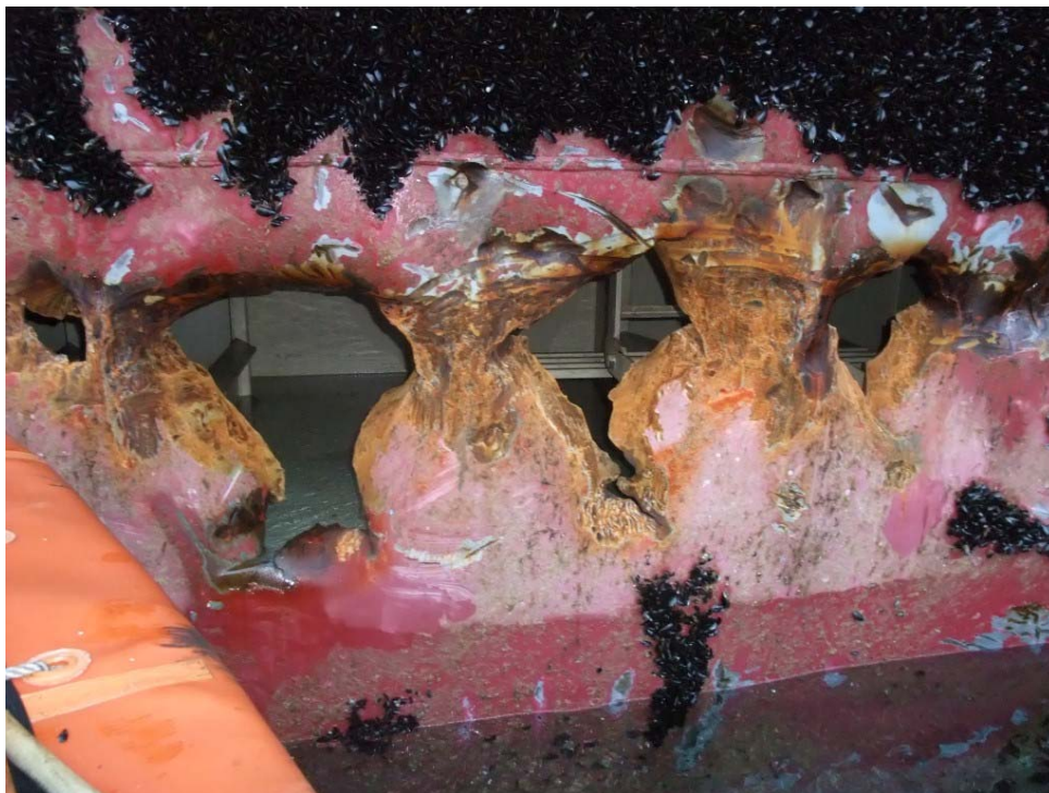
Figure 37: Five holes through the hull into tank 10. Note the clear marks from repeated blows. The hull between the holes is stiffened on the inside of the tank, and these stiffeners (about 0.6 metres apart) have absorbed the anchor's blows and prevented deeper intrusion to the tank's inner bulkhead (1.5 metres in). The photograph was taken in Kristiansund on 12 November 2012 by the PSA..
