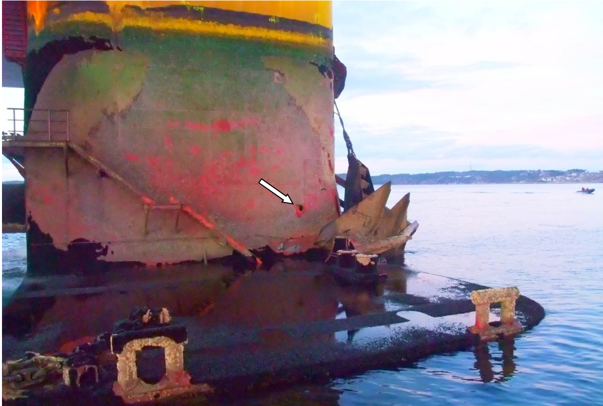
Figure 40: The forward port column on arrival in Kristiansund on 10 November 2012. Anchor 8 is wedged in the bolster and the hole into tank 10 (arrowed) is clearly visible. Some scrape marks at the bottom of the column show that the anchor has moved in the area. The pennant wire twined around the anchor line (above the anchor) shows that the anchor has rotated. The photograph was taken by the PSA.
