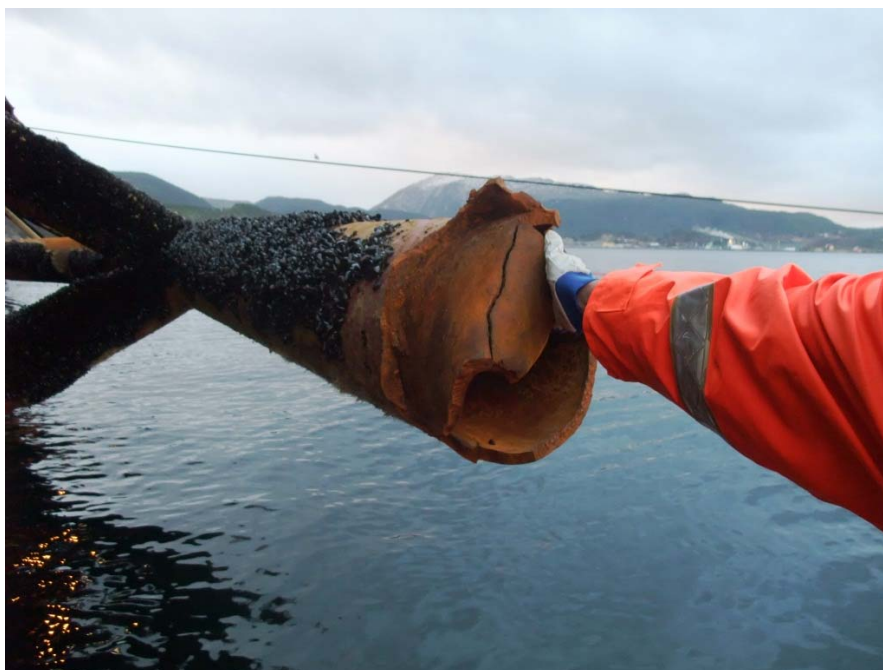
Figure 29: Bolster 4 with damage A (see Figure 27). Three components are missing at this point. The first fracture on the incident night is assumed to have occurred here at 23.40 on 6 November, when overload alarms on the anchor winch ceased. Until then, the anchor could have pulled with a load of 70-80 tonnes in the horizontal bolster bar A-B (see Figure 27). The fracture has developed from the earlier damage, which is thought to have occurred in the lower brace (see Figure 28). This fracture caused a reduction in the anchor load, and allowed the anchor to start moving. The bolster bar between A and B may have remained for a time. After about two hours, the anchor has been able to hit the hull. Before that, the bolster has suffered yet another weld fracture at B and the bar – weighing about 1.5 tonnes – has fallen to the seabed. Both braces have been present until 01.40, with the upper probably still attached to point B (where the hand in the photo is holding a component which was bent after 01.40). The photograph was taken in Kristiansund on 12 November 2012 by the PSA.
