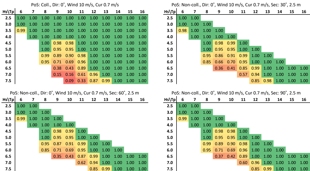
Figure 6: Drilling-rig results for a following-sea heading (0°) at U_{10} = 10 m/s and U_c = 0.7 m/s. Top left: Collinear. Others: Non-collinear with secondary wave ( H_{s,sec} = 2.5 m) at relative angles of 30°, 60°, and 90°.
